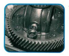
Here's a better view of a damaged retainer cup. Once the pinion shaft has eaten through the cup as it's done here, centrifugal force throws the pin out far enough for it to come in contact with the case. You can see all the aluminum chips thrown up as the shaft ate at the case.
