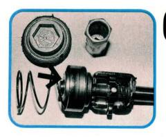
If the trans won't shift to neutral, you'll have to remove the selector in pieces. Carefully remove the snap ring on the retainer cup. We repeat, be careful! There's an even bigger, even badder set of springs in there that will send the cap and snap ring into never-never land. Trust me on this one.
