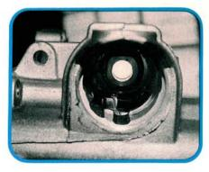
Remove the selector lever. Check the shaft seal at the opposite end of this hole for damage or heathardening. Replace if necessary. See how all the selector fingers are aligned? That's neutral. The finger closest to you is reverse. Remember that, we'll need it in a few moments.
