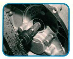
Remove the clutch push rod from the mainshaft. Bolt a bar across the bell housing that has an adjustable center bolt to support the mainshaft. Insert a spacer (copper or brass) between the end of the mainshaft and the adjusting bolt. Turn the bolt and spacer in until they just contact the end of the mainshaft.
