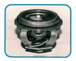
Remove the fifth gear synchronizer assembly. Then you can remove the four 5 mm internal hex head bolts directly beneath it that hold the clamping plate to the trans case. Also remove the circlip, washer, and fifth gear from the pinion shaft. You'll probably need a gear puller to remove fifth gear.
