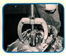
Whenever you replace a final drive housing, ring/pinion, or pinion bearings you'll need to check and adjust the pinion bearing preload. Preload is adjusted by changing the thickness of the shim beneath the lower pinion bearing race. Start by removing the bearing race with a set up like this.
