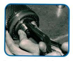
Remove the rear input shaft snap ring, then press off the fifth input gear and synchronizer hub. Inspect the parts for wear. The synchronizer hub and coupling sleeve are machined on both sides, although only one side is used for fifth gear. Flip both parts over to use the fresh side.
