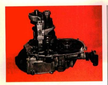
they have for any other reason. The impact from a minor front end collision can transfer through the transaxle mounts and crack the case housings. Off road excursions and close encounters with large boulders will also do expensive things to the aluminum castings.
