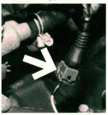
You can save time if the car you're working on is equipped with a cold start injector. Disconnect the harness connector at the thermo-time switch. (On this TCCS equipped Toyota Camry it's a brown connector, so don't confuse it with the
