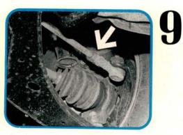
The front strut suspension allows for toe adjustment only. Loosen the lock nut and rotate the inner tie rod. No camber or caster adjustments are provided. If readings are out of spec, replace bent or worn parts. A nonadjustable three-link U-beam axle connects the rear wheels.
