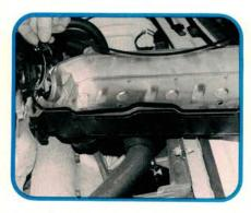
Clean the valve cover surface and groove before inserting a gasket in the cover. A little unwanted dirt will leave you with a leaky gasket. Check the gasket for cracks or wear; replace it if you have any doubts. We reused this gasket on our brand new car.
