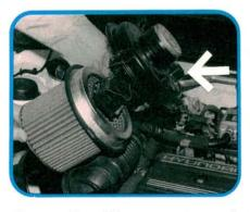
Remove the wiring connector and release three clips to remove the air filter housing lid. Be careful not to damage the air flow sensor located inside the filter itself when removing the lid. A dry type filter cartridge is serviced every 30,000 miles.
