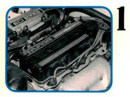
The Sonata uses an inline four-cylinder engine as standard equipment. Like the old 2.6 Mitsubishi engine, it has an overhead camshaft, two balance shafts, and a jet valve for each cylinder. The optional V6 engine has a belt driven camshaft in each cylinder head, but has no balance shafts or jet valves.
