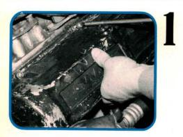
Most engine service procedures start with "disconnect the battery". It's especially important here. You could end up pulling the engine to replace the timing chain if the crankshaft turns during the later steps of a Saab "B" engine valve adjustment. Remove the spark plug wiring, crankcase breather hose, and valve cover.
