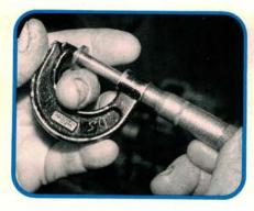
Measure the thickness of the original adjusting shim with a micrometer. Either add or subtract the number you marked on your chart to the thickness of the original shim. This gives you the correct thickness for the new adjusting shim.
