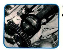
Saab recommends placing the transaxle in third gear, then rolling the car forward or backward to check valve clearances. Using a wrench to turn the cam boss while the cam sprocket is still attached may stretch the timing chain. A remote starter switch will do the job safely on stick or automatic models.
