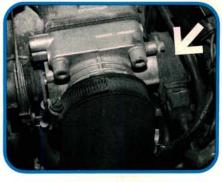
The Throttle Position Switch monitors throttle opening from its perch on the side of the throttle housing. Many throttle switches contain a set of closed and wide-open throttle contacts. The Throttle Position Switch sends an open circuit signal to the ECU when the throttle opening is between these points.
