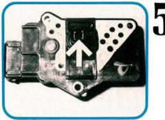
Nissan's Electro-Injection (EI) throttle body injection systems use a small hot wire Air Flow Meter. A passage directs an air sample around the throttle plates and past the Air Flow Meter. The Air Flow Meter sends its resistance signal to the ECU, which determines the total air flow based on the small sample.
