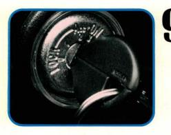
The ignition switch sends engine "start" and "on" signals to the ECU. The ECU uses these signals to control the Fuel Pressure Regulator, the Auxiliary Air Regulator, EGR operation, idle speed, ignition timing, fuel enrichment, and fuel pump operation.
