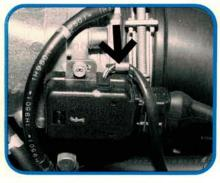
The Throttle Position Switch may also contain a potentiometer called a Throttle Sensor. The Throttle Sensor helps the ECU determine the actual throttle opening and how quickly the throttle position changes. In some ECCS systems, this sensor input helps the ECU control fuel shut-off during closed throttle deceleration.
