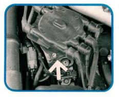
The Crank Angle Sensor uses a combination of photo diodes, LEDs, a shutter wheel, and a wave forming circuit inside the distributor to send crank angle and RPM signals to the ECU. The ECU uses the crank angle signal to control injector pulse duration, ignition timing, and other outputs.
