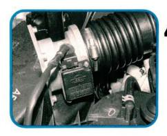
Since 1984, some Nissan models have been equipped with "hot wire" Air Flow Meters. The air passes over a heated wire after entering the air flow meter. The air cools the wire and causes the circuit resistance to decrease. The ECU converts the changing resistance signal into a measurement of the inlet air flow.
