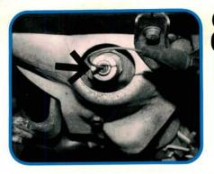
The oxygen sensor gives the ECU an indirect measurement of the air/fuel ratio by measuring the amount of oxygen present in the exhaust gases. You'll find heated (three wire) and unheated (single wire) oxygen sensors on different models. Sensors are usually mounted in the exhaust manifold.
