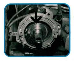
Three hundred and sixty slits in the shutter wheel tell the ECU how fast the engine is turning. Larger slots are used to signal crankshaft position. The largest slot indicates TDC for the number one cylinder. This is no place for dirt, oil, or stray light.
