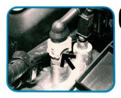
The Coolant Temperature Sensor contains a negative temperature coefficient (NTC) thermistor. Its resistance decreases as engine temperature increases. The ECU's 5-volt reference signal returns to the ECU at its lowest value when the engine is cold, and at its highest when the engine is warm.
