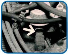
The Fuel Temperature Sensor measures fuel rail temperature from its position in the Pressure Regulator. The ECU monitors the sensor's signal, and increases the injector pulse duration when fuel temperature rises. This sensor is especially helpful in preventing hot restart problems.
