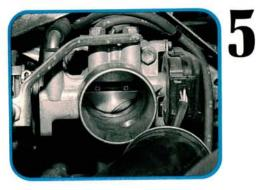
Loosen the clamp, then pull the inlet hose off the throttle housing. A deposit buildup on the inside of the housing can cause the throttle to either stick open or bind. A heavy buildup usually means PCV or blowby problems. Clean out the housing with carburetor cleaner, then lube the throttle bushings.
