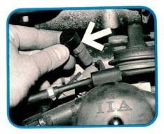
The green connector (arrow) at the base of the distributor gives an RPM signal for idle speed adjustments. Make sure your tachometer is compatible with Toyota's IIA. Refer to the December 1989 Import Service for detailed information on diagnosing Toyota IIA distributors.
