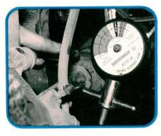
The ribbed drive belts used on Camry four cylinder engines may feel loose even when properly adjusted. Use a belt tension gauge to avoid overtightening, and prevent noise and premature wear. Toyota claims the belts will last 60,000 miles. We found a slightly frayed power steering belt that made it past the 100,000 mile mark.
