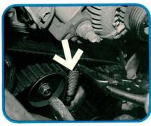
Timing belt tension is set by this spring (arrow). A loose belt will rub the inside of the plastic timing cover and may make a noise that sounds similar to a bad water pump bearing. Check the belt for wear, then loosen the idler pulley bolt. Turn the engine over twice, then re-torque the pulley bolt.
