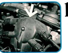
Electronic ignition, fuel injection, and hydraulic valve lifters take most of the meaning out of the words "tune up." All four spark plugs are easy to reach at the front of the 2S-E engine. Toyota's Integrated Ignition Assembly (IIA) distributor (arrow) is driven off the center of the camshaft.
