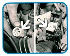
Stored trouble codes are retrieved from the ECU by jumpering this diagnostic connector (left photo), below the air flow meter ducting. The ECU blinks stored trouble codes on a dash-mounted check engine light. Later Camrys (right photo) use a more sophisticated self-diagnostic system and connector.
