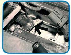
Maybe you're wondering, "How do I set the timing?" Well, you've got three choices. The cheapest method is to insert a short piece of secondary ignition wire between the number one coil and spark plug. Clamp your inductive timing light over the temporary plug wire and check the timing. Pretty low tech.
