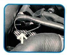
This wire loop at the Power Transistor Assembly is meant for an inductive tachometer hook-up. Depending on your timing light's sensitivity, you might be able to use the loop to check the timing too. Check the timing using the temporary plug wire method first. We'll need the reading later to compare timing light pickup sensitivity.
