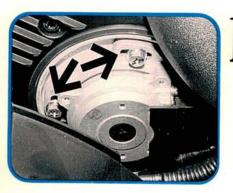
We'll start at the signal generating end of the Nissan ignition system. The "pancake" Crank Angle Sensor is driven by the nose of the 300 ZX's left exhaust camshaft. It's also driven by the exhaust cam on the Pulsar engine. The sensors on both engines are slotted for timing adjustments (arrows).
