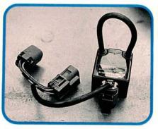
Our first method's biggest drawback is the amount of disassembly needed, especially on the Pulsar. A quicker answer is Kent Moore's dedicated Timing Coil. The Timing Coil connects between the Power Transistor Assembly and the number one coil to provide a temporary secondary wire for your timing light.
