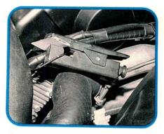
Place a folded match book cover between the pickup jaws. The match book prevents the pickup's pole pieces from contacting each other, decreasing the pickup's sensitivity. With luck, your timing light will now read the "off" signal. Now compare the desensitized pickup's primary reading to your original secondary reading.
