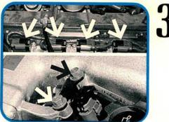
It takes some disassembly to reveal the ignition coils and spark plugs on the Pulsar (upper photo). They're hidden under a cover between the cam housings. Two bolts hold each coil on the 300 ZX (lower photo). A 60,000 mile spark plug replacement interval makes this job an occasional inconvenience.
