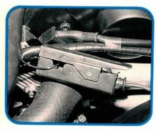
A sensitive timing light may pick up the power transistor's "on" signal instead of the "off" signal that fires the coil. If the light is triggered by the wrong signal at the loop, your light will blink about 15 degrees ahead of the correct reading. A cheap timing light can be an asset here.
