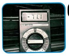
Observe correct polarity when you hook up your ammeter. With the key on and the engine not running, you should have a positive reading. If not, reverse your meter leads. Remember that plus readings mean a richer mixture is needed. You'll get negative readings when the differential regulator needs to lean the mixture, as in deceleration fuel cut-off.
