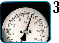
Close the valve on the pressure gauge. Leave the differential pressure regulator unplugged. The plate in the differential pressure regulator should deflect enough to give you a pressure differential between the upper and lower chambers. Pressures should be 0.3
