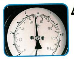
Reconnect the harness plug to the differential pressure regulator and crank the starter for about three seconds. This activates the regulator and sets differential pressure at its initial controlled operating pressure. Pressure should read approximately 1.3 to 1.6 bar below system pressure.
