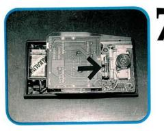
If the engine won't start after connecting the meter, check for loose connections or a bad meter. The meter is now in series with the ECU and the differential pressure regulator. An open circuit in the meter may stop the engine from running, or cause it to run very poorly. Our meter had a bad fuse, creating an open circuit.
