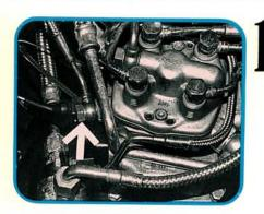
To check system fuel pressure, unplug the connector at the differential pressure regulator. Connect your gauge between the lower chamber test port (arrow) on the fuel distributor, and the line to the cold start injector. Open the valve on the gauge and run the fuel pump. This system runs at 6.1 to 6.5 bar.
