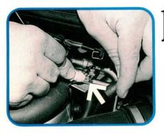
Check the oxygen sensor with the engine at normal operating temperature. Remove a vacuum line and watch for the mA readings to change. If the readings don't change, disconnect the oxygen sensor and ground the carside harness. If the readings change, replace the sensor and retest.
