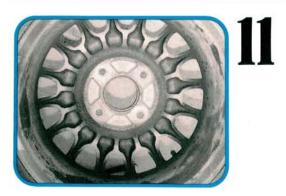
Honda techs suggested that stamped steel wheels distort more easily than these alloy wheels. They were also quick to note that an impact gun set at "twist off," will warp the alloy wheels as well. Make sure all corrosion and debris are removed from the inner face of all road wheels before installing them.
