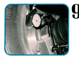
Since previously distorted rims or hubs can distort a new rotor, or ruin a resurfaced one, we want to make sure our freshly turned rotor will still turn true with the wheel in place. Here's one way to check. Temporarily install the wheel, but leave the caliper off. Tighten the lugs to specs. Mount a dial indicator as shown.
