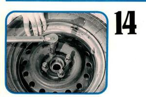
Bolt the wheel to the drum and recheck runout. If the wheel is warping the drum, reindex the drum and wheel and check again. Still no luck? Replacement of the road wheel may be the only lasting cure. Turning the drum/wheel as a unit may eliminate the runout, but it's dangerous, and that warped wheel will cause problems after the next tire rotation
