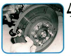
Measure the rotor and compare your measurements to minimum thickness specifications. If the rotor is thick enough to resurface, continue measuring with your micrometer at four equally spaced places around the rotor. We're checking for uniform rotor thickness or parallelism.
