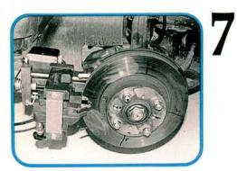
Machining rotors on the car trues the rotor surface to the drive hub. If a car has returned to your shop with a repeat case of judder a short time after its last brake job, simply replacing the rotors again is risky business. You may need to skin cut the new rotor on the car to true the assembly components and eliminate the runout problem once and for all.
