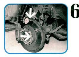
If the car showed up with overtightened lugs, the drive hub may be distorted. Try this test. Match mark the hub and rotor where you got your highest reading. Remove the rotor, turn it 90 degrees, and reinstall the lugs. If the dial indicator reading is the same, but the location moves 90 degrees, the rotor is the culprit, not the drive hub.
