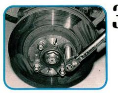
Check for looseness in the front suspension or wheel bearings. Check the tires for uneven wear or ply shifts. Then remove the wheel. Install and torque the lug nuts to hold the rotor tight against the hub. Check and adjust the steering rack tension if needed. While a loose rack may not cause judder, it will make it more noticeable.
