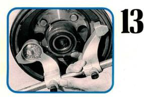
For cars with four-wheel discs, the test procedures are the same, although conventional off-the-car refinishing seems adequate for Honda rear rotors. For rear drums, check the drum for overall diameter and runout using a brake drum micrometer. If drum runout is greater than 0.05 mm (0.002 in), resurface the drum to true it.
