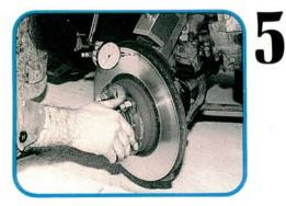
Measure the rotor face for runout using a dial indicator. Runout should be no more than 0.10 mm (0.004 in). Check for runout close to the hub, and near the edge. A rotor that passes this test with the dial indicator riding near the hub, may fail the same test as you move outward toward the edges of the rotor's braking surface.
