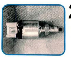
Another potential cause of brake overheating is an improperly adjusted brake light switch. Since Honda uses the brake light switch to set the upper limit for brake pedal travel, a switch that's screwed in too far can keep pressure on the pedal, causing the brakes to bind, heat, and warp.
