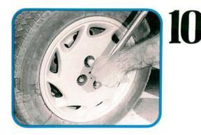
Checking the rotor with the wheel bolted in place tells us about assembly runout. If warped components are rewarping the rotor before it even leaves the shop, we're already in trouble. Look for a maximum 0.10 mm (0.004 in). If you're off by more than that, the source of the runout will have to be eliminated.
