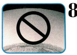
Honda recommends the Kwik Way lathe. Honda techs suggest that the best way to run the lathe is to block the opposite wheel and run the disc being turned at a speed of about 12 MPH with the lathe set on the medium or slow feed. This gives a nice smooth finish. Avoid the dreaded "record finish" at all costs.
