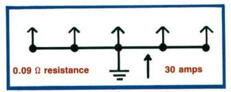
1) If a common ground connection has 0.09 ohm of resistance, and 30 amps is passing through it, what is the voltage drop measured by the DVOM?
