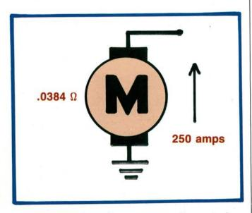
2) A starter motor draws 250 amps of current when cranking and has a resistance of 0.0384 ohm. How much voltage does the starter motor drop?
