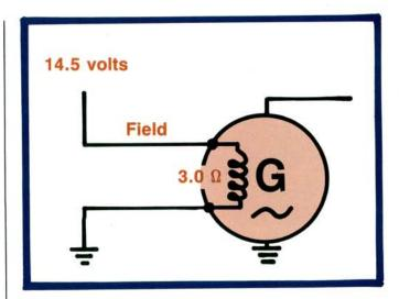
3) An alternator's field winding measures 3.0 ohms with a DVOM. How much excitation current flows through the rotor when the alternator charging voltage is 14.5 volts?
