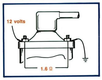
1) An ignition coil primary winding measures 1.6 ohms. How much current flows when the voltage applied is 12 volts?
