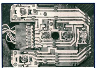
On 1986-88 Saab 9000s, there's a pictogram or safety monitor on the dash below the tachometer. The pictogram warns the driver of rear-light failures. But what if you replace a burned out rear bulb and the pictogram remains on? There's a good chance that the new bulb's resistance is substantially different from that of the other bulbs. Mismatched or corroded bulbs create an imbalance in resistance from the left side to the right side. The imbalance in resistance turns on the pictogram.
