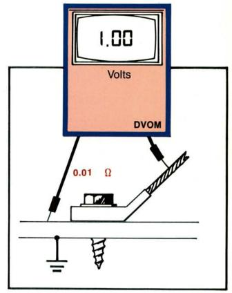
All it took was 0.01 ohm of resistance in a ground cable to cause a 1 volt drop (in this case a voltage loss) in a circuit with 100 amps flowing through it. You already know that a 1 volt drop in a circuit can cause big problems, and the resistance that caused this sizable voltage drop was too small to detect with your DVOM.
