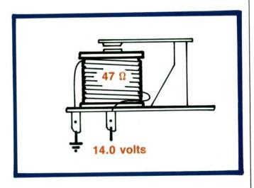
2) A relay winding measures 47 ohms. How much current flows through the relay winding if 14 volts is applied?
