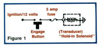
As you can see, the ''engage'' button is in series with a 5 amp fuse and the Hold-in Solenoid. The fuse blows each time the engage button is depressed. The resistance of the Hold-in solenoid measured 1.5 ohms with a DVOM. How much current is flowing through the circuit if the operating voltage is 12 volts?
