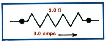
3) A ballast resistor is supposed to pass 3.0 amps of current in normal operation and it has 2.0 ohms of resistance. How much of a voltage drop should you measure across the resistor?
