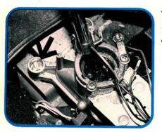
Removing the transmission shift cable can be a real battle on pre-1978 Saab 99s. We chose to remove the cable at the shifter end, then snake the cable through the firewall. It takes a little more time, but there's more room to work. A special socket is needed to remove the anti-theft shifter housing bolts (arrow).
