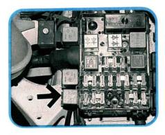
For safety's sake, the ECU powers the fuel pump through the fuel pump relay only when the engine is running at more than 300 RPM or during cranking. The ECU receives a voltage signal from the ignition switch during cranking and uses the engine speed sensor to detect minimum engine RPM.
