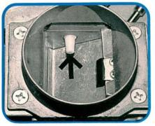
The air temperature sensor on the inlet side of the air flow meter helps the ECU decide the best air/fuel ratio and ignition timing over a wide range of temperatures. The air flow meter shouldn't be disassembled. If the sensor fails, the air flow meter must be replaced.
