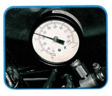
Fuel pressure normally runs in the 2.5 bar (36 PSI) range at idle. Since the ECU can't adjust the system to compensate for incorrect fuel pressure, begin any diagnostic work with a quick fuel pressure check. The system should also hold 2.0 bar (29 PSI) residual pressure for at least 15 minutes after shutdown.
