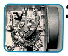
The ECU sends a constant reference voltage signal to the air flow meter. The air flow meter's potentiometer (arrow) returns part of the reference voltage to the ECU, converting engine load into a voltage signal that can be understood by the ECU. The voltage signal increases as engine load increases.
