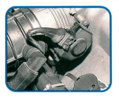
One set of throttle valve switch contacts is closed only at idle. A second set of contacts closes as the engine approaches full throttle. Both sets of contacts are open between these points. Switch position affects idle speed, timing, deceleration fuel cutoff, and full throttle enrichment.
