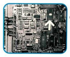
The ECU's computing circuits are mounted on a second circuit board. All of the ECU's maps are stored on one ROM chip (arrow). All input and output signals are digitally processed by the ECU at a clock speed of 6 Mhz. That's slow by computer standards, but plenty fast for automotive use.
