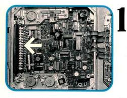
This dissected ECU shows you some of the more than 200 electrical components inside a Motronic ECU. A single 35 pin plug (arrow) connects the ECU to the battery, input sensors, and output devices. This circuit board holds the power output stages for the fuel injectors, ignition, and fuel pump.
