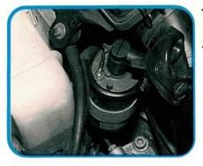
An output stage inside the ECU controls the ground side of the coil's primary windings. The ECU controls ignition timing and dwell functions at the coil with no intermediate step. The ECU also advances or retards the ignition timing to fine tune small changes in engine idle speed.
