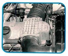
All intake air should pass through the air flow meter before reaching the engine. Any vacuum leaks (false air) will affect the accuracy of the air flow meter's signal to the ECU. The air flow meter adjusts for engine wear, valve clearance changes, compression changes, and intake valve or combustion chamber deposits.
