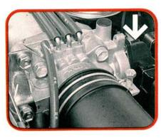
The throttle position sensor signals the ECU when the throttle is fully closed. When the throttle is opened, a potentiometer returns a varying voltage signal to the ECU, used by the ECU to determine throttle opening angle. Knowing the throttle opening angle helps the ECU determine the engine load.
