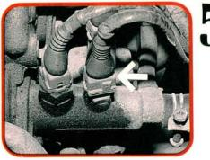
The coolant temperature sensor helps the ECU decide the correct amount of fuel enrichment needed as the engine warms toward operating temperature. The sensor's negative temperature coefficient (NTC) thermistor resistance is high when coolant temperature is low, and decreases as the engine warms.
