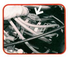
The distributor signals the ECU using its NE and G sensors. The NE sensor gives the ECU an engine speed signal. The ECU uses the G sensor signal (crankshaft angle) to help determine proper injection and ignition timing. Some distributors have two G sensors, giving the ECU two separate crankshaft angle signals.
