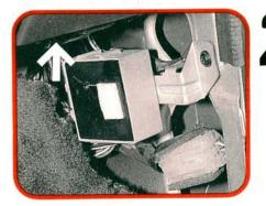
The twin coil circuit opening relay is hidden behind the glove box on this Camry (arrow). The relay controls the voltage supply to the fuel pump. During cranking, the relay's first coil is controlled by the ignition switch. While running, a switch inside the air flow meter controls the ground to the second relay coil.
