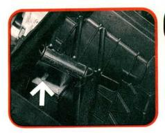
The NTC intake air temperature sensor sits in front of the air flow meter's potentiometer air flap. If the air temperature sensor fails, the ECU substitutes a resistance equal to a 65 degree F air temperature. The ECU can also substitute a coolant temperature value to keep the engine running if the coolant sensor fails.
