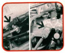
TCCS systems use a cold start injector to help out with cold engine starting. The injector's operation is controlled by the thermo-time switch and the ignition switch on most models. The ECU may also control the injector operation over a limited temperature range on some later systems.
