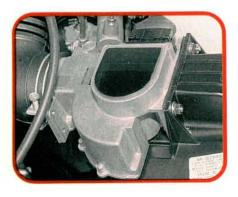
Most TCCS systems use an air flow meter to measure engine load. The ECU sends a 5 volt reference signal to the air flow meter. When intake air volume is small (low load), the air flow meter's voltage signal to the ECU is close to 5 volts. When intake air volume is large (high load), the signal voltage is close to zero.
