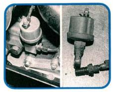
If you're installing the modified tensioners, replace the narrow, old style banjo fitting with the wider, square block. The new feed line is just a bit too short to reach the thinner, old style fitting. The line doesn't tighten properly, vibrates loose in a few thousand mile (or less), and leaks.
