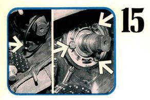
We also have some oil leaks to fix on this engine, so we'll remove the cam sprockets, and the three bolts in the camshaft retainer ring. With the retainer removed we found the o-ring behind the collar broken as shown. There's also a flat gasket between the retainer and camcase.
