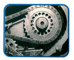
If the cam timing is way off, you'll have to loosen the retaining nut (or bolt), remove the lock pin, and turn the outer sprocket one full hole. If the reading is off only a tiny bit, there may be enough play between the sprockets and lock pin to loosen the nut and tweak the adjustment until it's in time.
