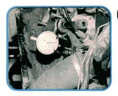
Valves adjusted? Check valve lift as shown. Attach a dial indicator holder to the cylinder head. The point of the indicator should rest on the upper valve spring retainer. Set the engine at TDC on number one. Preload the gauge for about 4 mm. Turn the engine 360 degrees in the direction of normal rotation.
