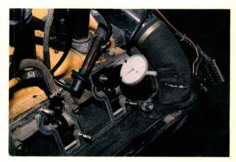
• What are we measuring when we measure camshaft timing? Maybe this illustration will help. What we measure is the TDC valve overlap. Our illustration shows sample intake and exhaust profiles.
