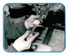
Before we remove the chains and sprockets, we need to make sure the faces of the intermediate shaft sprockets and cam sprockets are parallel. Remove the intermediate shaft cover. Measure from the casting face to the face of the intermediate shaft sprocket. Don't let the gauge hit the snap ring on the sprocket.
