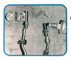
One caution: Starting in 1974, there was a modification made where the oil sending unit connects to the crankcase. A square junction block was installed with a threaded hole for the oil sending unit. On cars without a gauge, a threaded plug was installed in the junction block.
