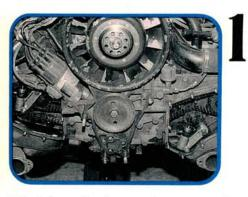
This job can be done in the car. You'll need to remove the rear engine hanger, sheet metal cover, and muffler. On A/C equipped cars, remove, but don't disconnect the compressor. Lay it off to the side. Then remove the timing chain covers and do a quick visual check for cracked or worn chain guides.
