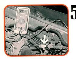
Check the throttle switch's IDL and E2 terminals for continuity at idle. A binding throttle linkage, or a misadjusted throttle switch may keep the switch contacts open at idle. The throttle switch should open when the throttle plate is opened approximately 0.025 inch.
