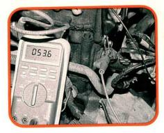
Hard starting problems after the car has been sitting in the sun for a few hours may also be traced to a faulty cold start injector time switch. The heat tricks the injector time switch into thinking the engine is warm enough to start without extra enrichment. Compare the switch terminal resistances to specifications.
