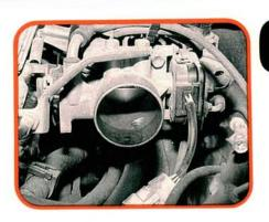
Carbon deposits inside the throttle housing can also cause the throttle plate to stick in different positions, giving the engine a different idle speed each time the throttle is closed. Remove the inlet hose, then clean the inside of the throttle housing. Lubricate the throttle shaft bushings with spray lubricant.
