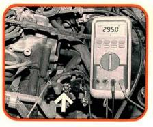
The coolant temperature sensor can lose its accuracy over time. The sensor still signals the ECU, but it may tell the ECU that coolant temperature is 170 degrees when it's really 190 degrees. Check the sensor's accuracy by comparing resistance values to specifications over a range of coolant temperatures.
