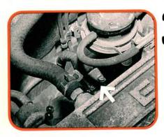
A clogged cold start injector (arrow) can also cause starting problems. The injector may become clogged if the car has been operated in a warm climate for an extended period. Remove the injector from the manifold, then trigger it with an auxiliary power source to check injector volume and spray pattern.
