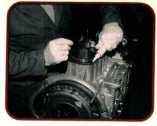
Lightly lube the thin green cylinder seals. Here we are applying the sealer to the flat face of the rubber seal. Install new sealing rings in the cylinder heads. Hold the sealing rings in the heads with petroleum jelly to keep them from falling out. We're almost ready to reinstall the heads.
