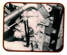
Before we can remove the piston/cylinder assemblies, we have to remove the crossover pipe and coolant flange. After positioning the pistons in the coolant flange opening, we will remove the piston pin retainer clips and piston pins through the hole. On the left side, we remove the water pump to access the clips and pins.
