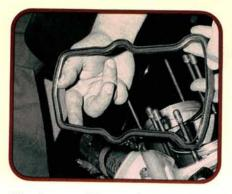
The large rubber gasket between the crankcase and cylinder head is grooved where it fits against the crankcase. This gasket does require a sealant (VW P/N D 000 400). Apply a thin bead of sealer on the flat face of the gasket facing the cylinder head. No sealant is needed in the grooved section facing the crankcase.
