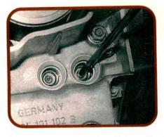
You can't see the lifters this well with the push rod tubes installed, so this photo was taken without the push rods tubes. Don't count on the push rods finding their way to the centers of the lifters. As you install the rockers, spin and wiggle the rods until they're properly centered in the lifters and rocker arm sockets.
