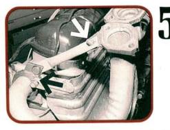
More potential confusion. Notice the "layered look." The exhaust slips onto a stud on the head, the mounting ear on the metal shield below the push rod tubes fits over the exhaust flange, and a support bracket acts as an outrigger for support. During reassembly doing things in the wrong order means doing them over.
