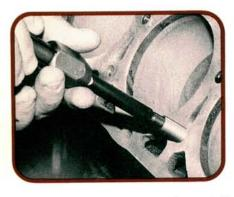
The threaded inserts used are different from those found in a regular Helicoil kit. They are 21/2 times longer than the diameter of the head bolts (equal to 14 threads). Install the inserts with the Helicoil installation tool. A small dab of Loctite is recommended. The coil pilot link can stay on the insert.
