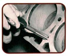
Now finish-cut the threads with the Helicoil tap to a depth of 35 mm. Once again, make sure the tap is properly lubed, and blow out ALL the chips. Rethreading kits are available from Benz in kit form P/N 900 589 00 99 00. Generic drills and taps of the correct size will work, however.
