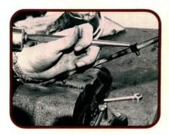
Replace all of the plastic inserts on the cam lubrication tubes (P/N 116 180 0184). Place the tubes in a vise to hold them. Use a small punch and hammer to tap the inserts one at a time along the length of the tube until each one pops off the end. New inserts can be installed by hand.
