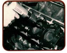
When we said a "properly sharpened" bit we meant it. Improperly sharpened bits will cut oversized holes. Badly worn bits may cut undersized holes. The final drilled diameter should be at least 10 mm but no larger than 10.3. Holes that are either too small or too large will give us weak threads.
