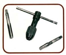
Pre-cut each thread with a pilot tap. Lube the tap with honing oil. Use a T-handle and tap by hand. Back off the tap a quarter turn or so if you feel the tap begin to bind as chips build up. When you're done, blow out the chips with compressed air. Wear approved safety goggles!
