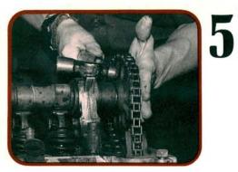
Remove the sprocket bolts (one on each cam) and the sprockets. Let the chain drop into the front cover. This may send a chill down the spines of old Datsun techs, but don't worry, there are no other tensioners to pop out. You can fish out the chain later with a hooked tool or piece of wire.
