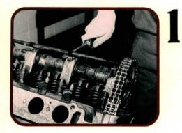
With the engine mounted on a stand, set the engine to TDC on number 1, and remove the valve covers. Make sure you have a good set of metric hex sockets in both short and long versions. Cam lubrication tubes can be removed by prying under the plastic inserts with a suitable tool.
