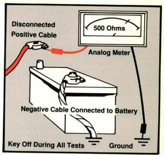
Dividing the battery's 12.6 volts by the electrical system's 500 ohms of resistance tells us that the key off battery drain is 0.0252 amps (or 25.2 milliamps). This key off battery drain is too small to cause any problems.
