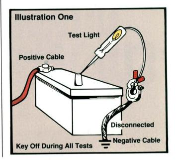
Another old time method was to place a voltmeter in series with the same battery terminal and cable we used for the test light. This method worked pretty well when we were still using analog voltmeters that had 1000 ohms per volt input impedances. The voltmeter would read about six volts if there was a key off drain problem.
