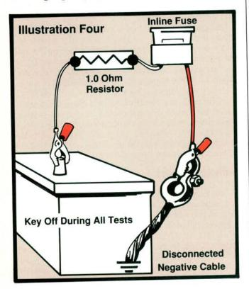
You'll need to buy an extra set of test leads for your DVOM, a 1.0 ohm/10 watt resistor, and an in-line fuse holder. Cut the positive test lead near the test probe, then solder the in-line fuse holder in place. Now solder the resistor between the test leads as shown. Protect the solder joints with tape or shrink wrap tubing. The resistor can even be enclosed in a small project case if you want to get fancy.
