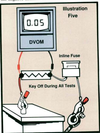
We're showing 0.05 volts on our voltmeter in this example. We'll use Ohm's Law to figure the actual amount of key off battery drain, measured in amps. Multiply the 0.05 volt reading by 1.0 ohm (the voltage drop across our 1.0 ohm resistor). Now we know that key off battery drain is 0.05 amps, or 50 milliamps.
