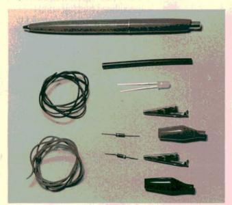
3 Now we'll get fancy. This battery powered LED test light tells you whether you're probing a negative or positive voltage source. You'll need two 1250 ohm ¼ watt resistors, two color-coded alligator clips, a 2 volt two-color LED, heat shrink tubing, a ball point pen body, and light gauge wire.
