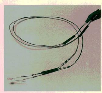
4 Solder the resistors, alligator clips, and wiring together as shown. Then solder the free end of the wire to the shorter, cathode leg of the two-color LED. Protect the solder joints with heat shrink tubing. We'll hook the two alligator clips to the battery when we're ready to use the test light.
