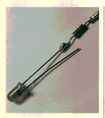
To make the LED test light, you'll need a 2 volt LED, a ¼ watt 1250 ohm resistor, wire, shrink wrap tubing, and two color-coded alligator clips. Solder one end of the resistor to the shorter, cathode leg of the LED. Solder a length of wire to the resistor's other end. Use heat sinks while soldering.
