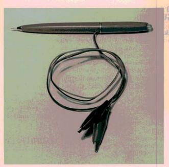
5 Solder the LED's longer anode leg to a large needle or other pointed object. Use the tip for probing wiring terminals and connections. Enclose everything in the pen body, with the two color LED at the top and the test probe at the bottom. Feed the battery leads through a hole in the side of the pen.
