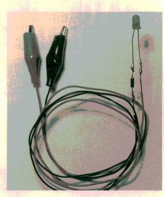
2 Solder a matching length of wire to the LED's longer, anode leg. Cover your solder joint with heat shrink tubing. Now solder the black (negative) alligator clip to the cathode wire and the red (positive) clip to the anode wire. Always observe proper polarity when testing circuits.
