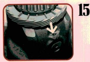
It's a good idea to remove and replace the differential spider gear shaft roll pin (arrow) during an overhaul. These pins have been known to break, which lets the spider gear shaft slide out of the spinning differential housing. A loose spider gear shaft will really do a number on the inside of the transaxle case.
