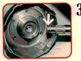
The inner pump bushings support the forward clutch shaft. A wobbling forward clutch will wipe out this seal (arrow) at the tip of the overdrive unit's intermediate shaft. The leaking seal keeps lube oil from passing through the forward clutch to the overdrive unit. Lack of lubrication will cause overdrive melt down.
