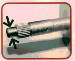
Many of the parts in the A140 are similar to parts used in other Toyota transmissions. Look for an extension at the tip of the forward clutch shaft (arrow) to identify locking torque converter versions. There's no o-ring seal, so any wear can cause fluid pressure loss and locking torque converter problems.
