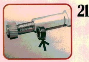
The transaxle case has separate fluid reservoirs for the transmission and differential. A leak at the speed-ometer gear seal (arrow) can drain the fluid out of the differential section and into the transmission. The transaxle will shift normally right up until the differential fails from lack of lubrication.
