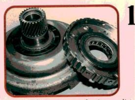
Pay careful attention to the intermediate sprag's installation direction. The sprag should turn freely in a clockwise direction when it's installed correctly. The whole transaxle will lock up when it tries to shift to third gear if the sprag is installed backward.
