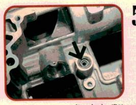
A backed out intermediate brake (B2) cup seal can cause second gear slippage on early A140s. The B2 cup seal is driven into the case to prevent pressure loss between the valve body and the intermediate brake. Don't forget to install this second seal (arrow) between the passage and the valve body.
