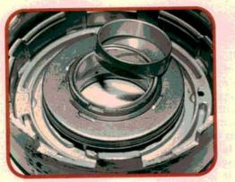
Early A140s used babbit-style bushings in the clutch drums and oil pump bushings. Worn babbit bushings are one of the main reasons early A140 transaxles fail. Later A140s have longer wearing bronze bushings. Aftermarket bronze replacement bushings are available to repair early A140s.
