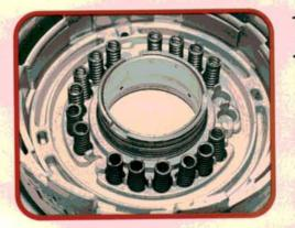
Keep a close eye on the number and location of the clutch drum release springs (we've already removed two here). Different length springs are used in each of the clutch drums. Either disassemble your clutch drums one at a time, or make sure you keep each set of release springs in a separate place.
