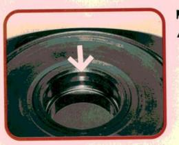
Check each clutch drum for wear in the area where the sealing rings ride (arrow). Dirty fluid combined with the Teflon sealing rings can wear grooves in the drum's sealing surface. High mileage transaxles may also show this wear, even with clean fluid. Clutch drum replacement is the only fix.
