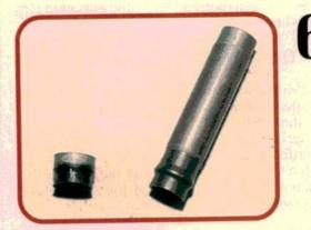
Later B2 seals (right) have an extension which reaches almost to the bottom of the valve body and prevents the seal from backing out. Some techs had problems with the early seal (left) because they installed it either too deep or too shallow. Both mistakes will cause pressure loss to the B2 circuit.
