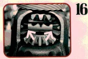
While you have the roll pin out, carefully inspect the spider gear shaft. Early, gray colored shafts may become worn in the area where the spider gears ride. Later models have a gold colored shaft which seems to hold up better. Gold shafts may be installed on early transaxles.
