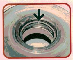
Measure the new sealing ring end gap before installation. Stretch the new seals by hand first, then place them inside the clutch drum in their installed position. Measure the seal's end gap the same way you measure piston ring end gap. Maximum allowable seal end gap is 1 mm (0.040 in).
