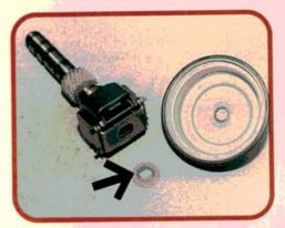
This nylon thrust bushing sits on top of the governor to keep the governor located in the case on A140L transaxles. If the bushing wears out or is lost during an overhaul, the governor will walk out of the case, gouging the governor cover and causing a loss of governor circuit pressure.
