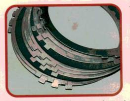
Different versions of this transaxle may have back-toback steel clutch plates (sometimes as many as three back-to-back) in different brake and clutch packs. The steel plates are used to help dissipate heat. Both overdrive clutch packs use extra steels to handle the extra heat in this area.
