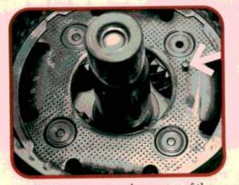
Small pins (arrow) at the center of the overdrive unit's planet pinions direct the flow of lubricating oil toward the pinions. If one of the pins falls out during an overhaul, the oil will leak through the open hole. No lube oil gets to the pinion and bearing, causing a planetary failure.
