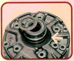
This plastic thrust washer at the back of the oil pump (arrow) controls overall transaxle end play. Only two shim sizes are available. So if you get the transaxle back together and the end play is wrong, you've probably got something assembled wrong. Check for proper installation of the thrust bearings and races.
