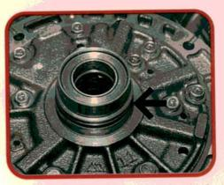
Also check all sealing ring lands for wear. Worn bushings or fluid contamination can round off or damage the ring lands' sharp edges. Sloppy ring lands can make for loose fitting Teflon sealing rings. Damaged ring lands can also keep the sealing rings from turning or sealing properly.
