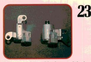
Intermittent operation of the electronic shift solenoids on A140E transaxles can cause strange shifting complaints. The solenoid electromagnets can also attract stray metal or may simply die of old age. When activated, the solenoids dump pressure, allowing the valve body shift valves to move.
