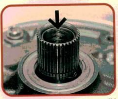
Worn internal oil pump bushings will let the internal transmission parts wobble as they rotate. This causes wear and fluid leakage in other parts of the transaxle further down the line. Worn pump bushings can cause the overdrive unit at the other end of the transaxle to fail, as we'll describe next.
