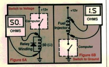
to the resistance of a known good relay. A low relay winding resistance could cause the computer's PNP switch to voltage circuit to fail. In Figure 6B, the resistance of a fuel injector is checked with a digital ohmmeter. Low resistance across the injector's winding can cause a switching circuit failure, this time in the NPN circuit.
