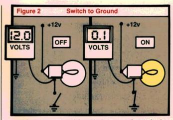
Voltage is available all the way through the filament of the lamp, and as a result, we can "see" it at the ground side terminal with our voltmeter. When the switch is closed, we have ground applied to the ground side of the filament. Circuit current begins to flow through the lamp which drops virtually all the voltage.
