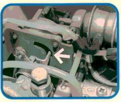
As you disconnect the assorted brackets to remove the carb top, remember that there's a bimetal choke spring hiding in that slot (arrow) in the choke housing. Later at reassembly, you'll need to use a small pick or hook to push the spring into position until it re-engages the choke lever.
