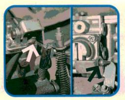
Remove the pivot shaft and arm from the accelerator pump housing to get at the fourth screw on the housing cover. Remove the E-clip (arrow) on the shaft and slide it out. Don't forget to reinstall the steel washers between the arm and pump cover. Accelerator pump overhaul is standard fare after that.
