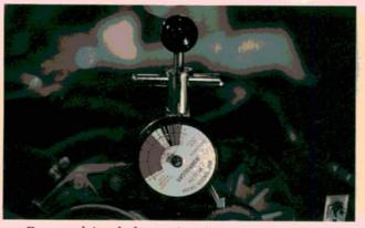
Proper drive belt tension is necessary to ensure quiet operation and maximum belt and bearing life. Borroughs Automotive Tools and Equipment offers a complete line of belt tension gauges, including the BT-33-73F shown here. This tool is calibrated for Asection V-belts as well as K-section poly V-belts, and covers a belt tension range between 130 and 800 Newtons (30-180 pounds). Timing belt tension gauges, as well as other tension gauges for specialized uses, are also available from Burroughs.
