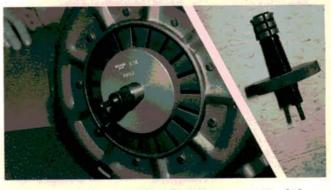
The model 6200 Clutch Alignment Tool from Assenmacher Specialty Tools assures proper clutch disc alignment during clutch service work on virtually all manual transmission vehicles. Two clutch mandrels supplied with the 6200 allow precise alignment of all clutch discs with internal spline diameters between 17.75 and 30 mm. Once assembled, the 6200 holds the clutch disc and pressure plate in proper alignment until clutch installation is complete. After installation, the tool can be easily removed.
