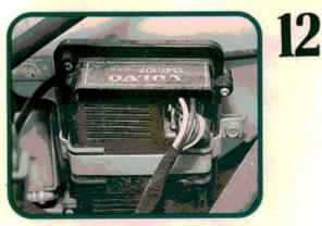
Ignition isn't controlled by the LH control unit. This separate control unit on the right inner fender handles the spark control duties. The LH control unit uses a signal from the negative side of the coil primary as a main sensor input. Later LH-Motronic systems combine fuel and ignition control.
