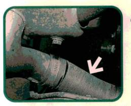
Check the operation of the thermostatically controlled air filter housing during each 5000 mile service. A defective thermostat will direct heated exhaust manifold air (arrow) through the air mass meter at all times and may cause premature air mass meter failure. If the air mass meter has failed, check the thermostat.
