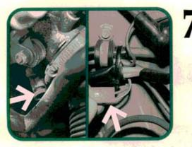
Base idle speed is adjusted at this thumb screw under the throttle housing (left photo). Before setting base idle, ground the blue/white wire in this two wire connector below the ignition coil (right photo). The throttle plate and throttle switch must be closed during this adjustment.
