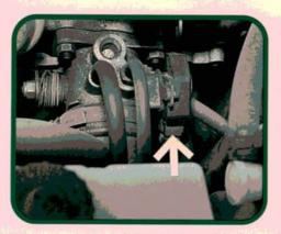
The throttle switch has idle and full throttle contacts. Both sets of switch contacts are open when the throttle opening is anywhere between these points. The switch's closed throttle contacts should click open as soon as the throttle is opened. Check switch contact operation with an ohmmeter.
