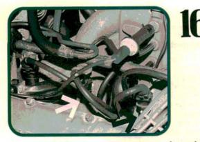
Check for leaking injector o-ring seals and intake manifold gaskets on high mileage engines. Any extra unmeasured air that sneaks in will affect system operation. Spray the areas around the injectors and intake ports with carburetor cleaner while watching for changes in the idle speed.
