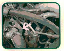
The coolant temperature sensor is near the thermostat housing and easier to reach on late model 240s. The negative temperature coefficient (NTC) sensor's resistance should be 290-364 ohms at 80 C (175 F). High sensor resistance readings at the ECU may be caused by a poor sensor ground at the intake manifold.
