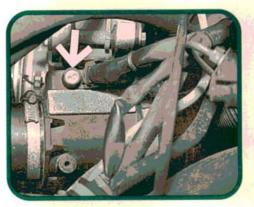
To adjust CO percentage, disconnect the oxygen sensor, then remove the anti-tamper plug at the air mass meter (arrow). If you can't adjust the CO to specs, check carefully for vacuum leaks, a misadjusted throttle switch, poor connections to the air mass meter, or a failed air mass meter.
