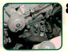
Deposits in the throttle housing may keep the throttle plate from closing completely at idle. This can also keep the throttle switch contacts open, which will raise the idle speed about 300 RPM above normal. Remove the air inlet hose, then use carburetor cleaner to remove the throttle housing deposits.
