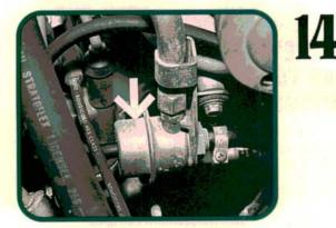
The fuel pressure regulator's vacuum diaphragm (arrow) maintains the fuel system pressure at aconstant level above intake manifold pressure. Several shops suggested to us that bad pressure regulators are the cause behind many fuel pump failures. Always check the regulator's operation when you replace a pump.
