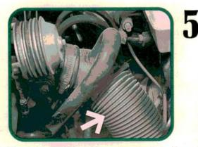
Check for vacuum leaks in the plastic bellows that connect the air mass meter to the throttle housing. Bellows leaks allow false air into the system, causing a rough, unstable idle, and sputtering during acceleration. These symptoms are similar to air mass meter problems. Check the bellows before condemning the meter.
