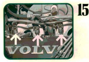
All four injectors fire at once. Injector pulse duration is controlled by the ECU. Connect an ohmmeter between fuel pump relay terminal 87 and ECU terminal 13 to test the injector circuit resistance. Total circuit resistance should be about 4 ohms. Higher resistance indicates defective injectors or injector wiring.
