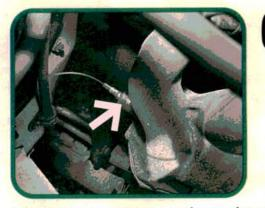
A hesitation at cruising speeds may be caused by a contaminated or lazy oxygen sensor (arrow). The oxygen sensor's switching time will slow as it gets older. Switching time can be tested with an oscilloscope. An alternate method is to disconnect the sensor, then drive the car to see if the hesitation disappears.
