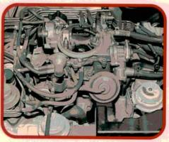
A cold stall or rough idle cold problem may be caused by a leaking carb base insulator block. Honda suggests checking the bases by spraying carb cleaner at the base. If the added enrichment keeps a cold engine running, the base is leaking. A new, improved base is available from Honda to cure the problem.
