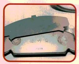
Some techs said they have to sell the added cost of OE brake pads, but most swore by the kits for sure stops and no noise. The kits include hardware, backing plates for the pads, and a bag filled with Molykote M 77. Apply the paste to both sides of the backing plates to further reduce chances of noisy brakes.
