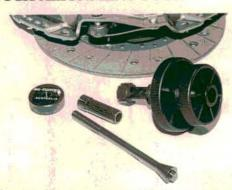
The All Clutch™ clutch aligning tool from Durston Manufacturing Company allows the clutch disc and pressure plate to be assembled and aligned away from the vehicle. This direct alignment allows a precise, mistake-free alignment on the workbench. Both plates are then installed as an assembled unit, eliminating the need for a third hand. The tool will fit all vehicles up to five tons with single plate clutches, and is manufactured of abrasion-resistant nylon.
