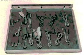
The 2800 Ignition Coil Adapter Kit from Mac Tools includes 13 different ignition coil adapters to fit most import and domestic ignition systems. The test adapters are connected between the coil and coil wiring harness, allowing for convenient hookup of tachometers and other test equipment. All adapter connectors are designed to prevent hookup errors. Complete instructions are furnished and all adapters are stored in a durable plastic case. Coil adapters are also available separately.
