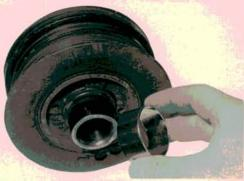
Dirt caught between the harmonic balancer and seal can wear a groove in the balancer's polished sealing surface. Installing a new seal over a worn balancer is an open invitation for a repeat oil leak. Fel-Pro's Sleeve and Seal™ Repair Sleeves offer an alternative to harmonic balancer replacement. The repair sleeve slides over the worn balancer surface, and is held in place by an anaerobic sealer. Nine part numbers provide repair sleeve coverage for domestic and import cars and trucks.
