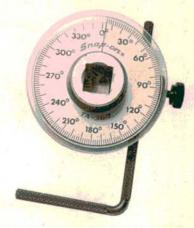
Many manufacturers now specify a torque angle sequence for their critical bolt tightening measurements. Snap-on's TA360 Torque Angle Gauge takes the guesswork out of these procedures by accurately indicating the number of degrees the fastener has turned on a large, easy to read scale. The gauge features a 360 degree scale with 2 degree increments, as well as larger 10 and 30 degree intervals. An adjustable arm holds the scale stationary during torque angle measurements.
