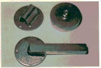
These specially designed floor jack adapter plates from Automotion provide a convenient way to lift a wide variety of Porsche models. The jack plates fit into the standard jack socket location, saving rocker panels and floor pans from dents. The round head on each jack plate is designed to rest securely on a hydraulic floor jack lift pad. Automotion's three floor jack adapter plates will safely lift Porsche 356, 911, 912, 914, 924, and 944 models from 1965 to current models.
