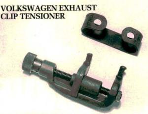
Removing the front exhaust pipe on a gas or diesel engine Volkswagen Rabbit, Golf, or Jetta, can be a dangerous experience. This exhaust clip tensioner from Baum Tools Unlimited uses a heavy duty screw thread and square drive to safely expand the large spring steel exhaust retaining clips during exhaust pipe removal. The tool takes the place of the wedge set that was previously recommended for this job. Baum Tools offers a complete line of factory and specialty tools for imported vehicles.
