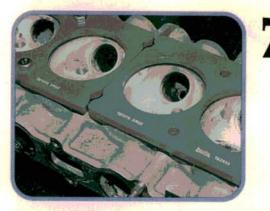
These special fixtures seal the head's external cooling passages so the head can be pressure tested. All core plugs must be tight when using this testing method. Slowly bring the pressure up to 50 PSI, then listen for leaks. Cover the head with soap suds. Small leaks will show up as soap bubbles.
