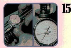
If you're planning to reuse the valve springs, measure their free height, straightness, and spring tension. Weak, twisted, or corroded springs should always be replaced. Our springs were slightly compressed and weak. At 100,000 miles, we decided to replace all of them.
