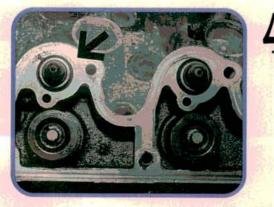
Two cam housings bolt to the top of the Toyota head. Head or cam housing distortion can cause the cams to bind. Check the mating surfaces on the head as well as the intake and exhaust manifolds and manifold mounting surfaces for warpage or damage. Toyota recommends replacement of any warped parts.
