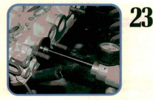
A Sioux vacuum tester was used to check for a good valve-to-seat seal before installing the valve springs. Each valve held at least 20 inches of vacuum. Proper sealing is important, a gap the thickness of a human hair between the valve and seat can cause leakage and loss of compression.
