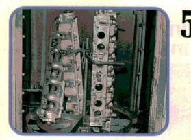
A jet washer and caustic soda removed most of the dirt. Later we glass beaded the head to remove deposits from the areas the jet washer couldn't reach. Make sure all left over beads are removed before reassembly. Thermal cleaning methods used for cast iron parts aren't recommended for aluminum castings.
