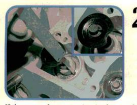
If the new valve protrusion is close to the original measurement, installed height should also be correct. Installed height is hard to measure on this head, so we ground a notch in a spare spring retainer of the same type. The vernier caliper fits next to the notch for an accurate measurement.
