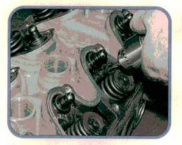
The Toyota's lash adjusters were wasted. Heavy sludge had clogged the adjuster oil drain passages, and the adjusters were stuck solid in their bores. We tried grabbing the adjusters with locking pliers, but they wouldn't budge. We drilled the drain passages to remove the sludge.
