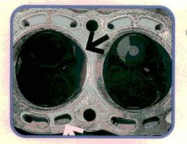
There are other problems besides warpage that may require resurfacing. Watch for erosion around the coolant passages caused by coolant leakage at the head gasket. Mild erosion can be corrected by resurfacing, if allowed. Also check for an undamaged head gasket sealing area around the combustion chambers.
