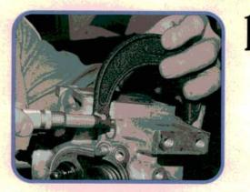
Start by measuring the head thickness. This will help you determine whether the head has already been resurfaced. There's no sense wasting time on a head that's already been machined to the limit. Some manuals list new and minimum head thickness dimensions. Build your own library of "known good" specifications.
