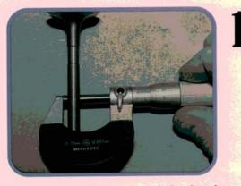
Measure the valve stem and check it for wear in the guide area. Compare the valve's overall height to specifications. Operating conditions can cause the valves to stretch over time. Wear in the keeper area is harder to measure. To assure a lasting rebuild, we replaced the valves and keepers.
