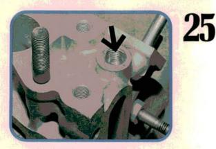
We drilled and tapped the oil passage openings to accept standard pipe plugs. Use a shop vacuum to suck the chips away from the head. Compressed air can blow chips back inside. All oil passage plugs were coated with sealer, installed, then ground flush with the head to prevent interference with other parts.
