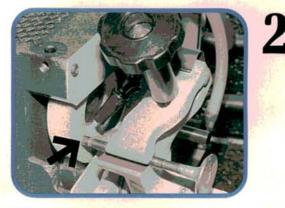
If the new valve stem protrusion is too great, it can be corrected by grinding a small amount of material off the valve stem tip using a valve grinding machine. Be careful here, we don't want to remove the valve tip hardening or cause interference between the valve spring retainers and the cam followers.
