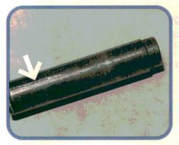
If the guides are removed without heating the head first, they will tear the aluminum head as they are driven out. This galled guide from a different engine shows the results. If new guides are also installed cold, the guide bores will be further damaged, causing a loose guide fit.
