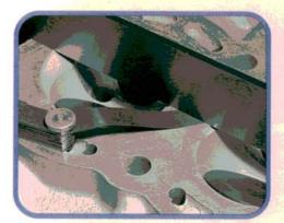
Clean the cylinder head sealing surface with a razor blade, then use a straight edge to check for warpage from several different angles. Toyota permits a maximum warpage of 0.10 mm (0.004 in) with no resurfacing allowed. We couldn't fit a 0.025 mm (0.001 in) feeler gauge under the straight edge.
