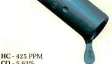
**CO** - 5.63%  $O_2$  - 2.3% (Since we have a miss, some of our oxygen is not being used. But remember,  $O_2$  isn't a really accurate indicator of a rich mixture—CO is telling us more in this case.)
