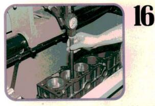
The finished cylinder dimension should be within 0.013 mm (0.0005 inch) for out-of-round and taper measurements. Some blocks require a deck plate during boring and honing. The deck plate simulates the stress caused by bolting the head to the block which may pull the cylinder walls slightly out of round.
