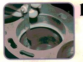
Use an inverted piston to square a ring in the cylinder bore to measure ring end gap. Toyota recommends ring replacement if ring end gap is incorrect (no filing allowed). Our cylinders were honed to a precise dimension so the rings fit perfectly without modification. Test fit the pistons to their bores.
