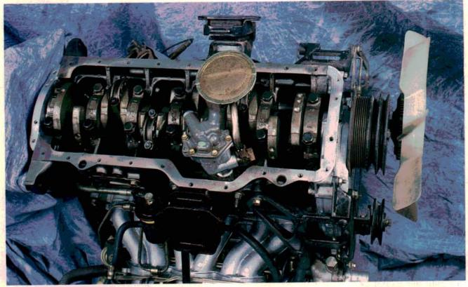
Last month we started our Toyota Cressida 5M-GE twin-cam six overhaul Head First with a complete reconditioning of the cylinder head and related components. This month we're ready to turn the Cressida's straight six Bottoms Up so that we can concentrate on lower engine inspection, overhaul, and assembly techniques.
