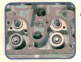
5M-GEs occasionally develop oil leaks between the cam housings and the cylinder head. Our aftermarket replacement gasket (arrow) was thicker than the OE paper gasket, and included an embossed sealing ridge to prevent oil leakage. We applied a thin coating of Hylomar to position the gasket during assembly.
