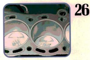
The slightly oversize sealing rings on this Fel-Pro head gasket will accommodate up to a 1 mm (0.040 in) cylinder overbore and chamfer. This design ensures proper clearance and prevents detonation or pre-ignition caused by the head gasket sealing rings protruding into the combustion chambers.
