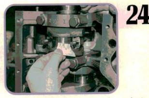
Lay a strip of Plastigauge across the crank pin, install the rod bearing and cap dry, then torque the rod cap nuts. Remove the bearing cap to check the oil clearance. Apply assembly lube to the rod bearing, put a dab of thread locker on the rod nuts, then retorque the nuts to specifications.
