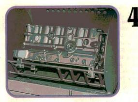
The block came out of the pyrolitic oven looking like it had been nickel plated. The oven heats the built up oil, dirt, and internal deposits and reduces them to a fine dust. Oven cleaning is a whole lot easier than the soaking and scraping routine that we're used to. Toxic waste is kept to a minimum too.
