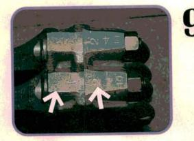
There are several numbers at the end of each connecting rod, but none of them refers to which cylinder the rod came out of. The number closest to the parting line refers to the selective bearing system (right arrow). Mark the rods and bearing caps with a punch for cylinder location (left arrow).
