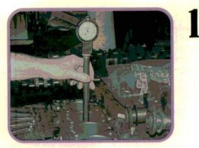
We checked cylinder measurements to make sure the block was rebuildable. We knew we had one damaged cylinder. Amazingly, the five remaining cylinders were practically unworn after 100,000 miles. Cylinder taper and out-of-round measurements were both within Toyota's 0.02 mm (0.0008 in) limit.
