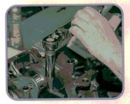
The new main bearing and crank journal should be clean and dry for an accurate measurement. Install the main bearing cap, then torque the bolts to specifications. Don't rotate the crankshaft during your measurements. Loosen the bolts, then carefully remove the bearing cap.
