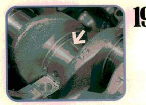
Install the crankshaft and bearings. Pay attention to the location of any special bearings or oil holes. The back side of the new bearings and the housing bores in the block must be clean and dry. Lay a strip of Plastigauge across the crankshaft journal to measure the oil clearance (arrow).
