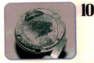
The pistons must be heated in hot water to 60 degrees C (140 degrees F) for piston pin removal. If you're reusing the pistons, clean the ring grooves, then use new rings to measure the ring groove clearance. A 0.03 to 0.07 mm clearance is required on the top groove and 0.02 to 0.06 mm on the second groove.
