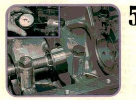
After torquing the main bearing cap bolts, we measured the housing bore diameters with a bore gauge to make sure they were all the same diameter. Toyota started a selective bearing system the same month our 5M-GE was built. Refer to the introduction to this article for a description of this system.
