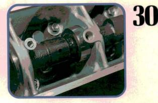
After installing the pan, we filled the engine with oil. Then for a final assembly check before installing the timing belt, we turned the auxiliary shaft pulley until the oil pump delivered oil to the cam lobe lubricating holes. We wanted these parts to get plenty of oil as soon as the engine started.
