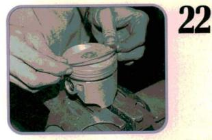
Install the new pistons on the connecting rods. Clamp the rods in a soft jawed vice, then install the new piston rings. These low tension rings slipped over the piston without a ring expander. Follow the manufacturer's recommendations for proper ring end gap positioning.
