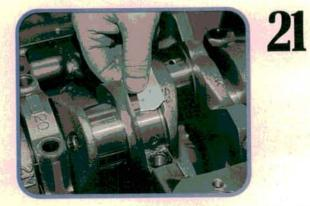
Our oil clearance was less than 0.04 mm (0.0016 in). Remove the crank and apply assembly lube to the main bearings and crank journals. All bearing cap bolts and bolt holes should be clean and lightly oiled. Follow the recommended bearing cap torque sequence. Make sure the crank turns freely and isn't binding.
