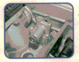
The oil pressure regulator (arrow) is a very important part of the upper engine lubrication system. We disassembled the regulator for cleaning and found the regulator valve was stuck solid. A stuck regulator will starve the upper engine for oil and will cause noisy lash adjuster operation.
