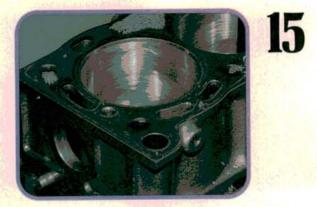
The crosshatch angle should be between 20 and 60 degrees. The smoothness of the cylinder wall finish is actually more important than the crosshatch angle. Use a 220 grit stone for finish honing with cast iron and chrome rings and a 280 grit stone for moly piston rings.
