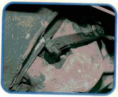
There's a cross shaft connecting the accelerator pedal to the external linkage pivot arm. This shaft can seize in the bushings, causing the linkage to stick and bind. Some get so rusted, that the linkage must be driven out of the old bushings before new bushings can be installed.
