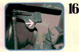
Remove the three bolts that attach the rear mount to the transaxle clutch housing. All three bolts thread into the left axle seal area of the clutch housing. Make sure you remove the correct bolts, since the upper half of the rear mount also supports the rear of the engine. Remove the stamped metal flywheel shield.
