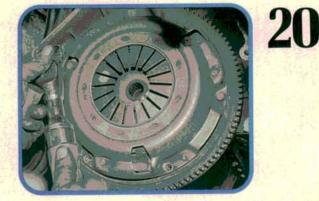
Give the new clutch disc a test fit on the input shaft. It's better to find out now whether you have the right disc. Use a clutch aligning tool to center and install the new clutch disc and pressure plate. Evenly tighten the pressure plate bolts to 26 Nm (19 ft-lb), then retrace the transaxle removal steps.
