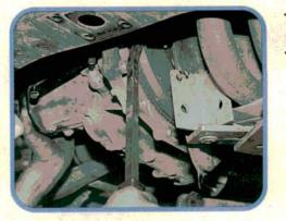
Push the transaxle away from the engine. The transaxle has a short input shaft and should clear the pressure plate. Use the weight of the differential to roll the rear of the transaxle downward as you lower the transaxle. This rolling maneuver lets the transaxle squeeze between the engine and right frame rail.
