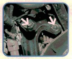
We're jumping ahead a little here. With the transaxle removed, you can see how the the torque arm bracket is attached to the transaxle. Two bracket bolts pass through the transaxle from the engine side, and one bolt comes from the transaxle side. Captive nuts in both bracket halves hold all three bolts in place.
