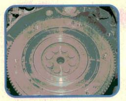
Remove the clutch disc and pressure plate, then inspect the flywheel surface. Some Honda techs recommend a flywheel refacing job with every clutch replacement to avoid chatter problems. If you're fixing a Blue Plate Special, the heat damaged flywheel may need to be replaced rather than refaced.
