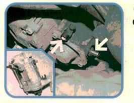
We pushed aside a tangle of emission hoses to get this photo of the starter. The starter motor's electrical connections are pretty easy to reach, its mounting bolts are not. The long upper mounting bolt passes through the transaxle to the engine. The shorter lower bolt threads into the transaxle.
