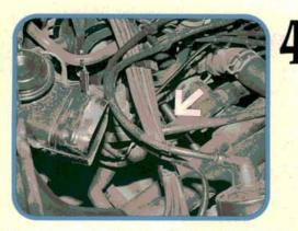
Disconnect the backup light switch wiring connectors located near the air cleaner assembly. Use an extension (arrow) to remove the two upper transaxle mounting bolts. The first is directly above the upper starter mounting bolt hole, the second is further forward. Eyes on your fingertips will help to find them.
