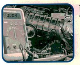
Check the adjustment of the throttle position switch. There are three pins in the TPS. Here we check for continuity between the left and center pins at idle. Then check from the center pin to the remaining pin for continuity at wide open throttle. Make sure to use your POZIDRIV<sup>™</sup> on the TPS retaining screws.
