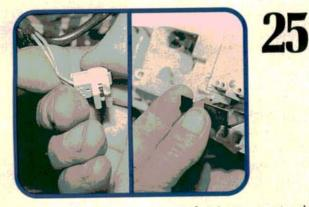
Back at the car, reconnect the instrument wiring. Replace all connectors (color coded). Push the main connectors squarely into their sockets and press down the locking tabs. Don't forget the small blue connector. It can be tough to plug in by feel alone. Push in the black locking slide over the plug.
