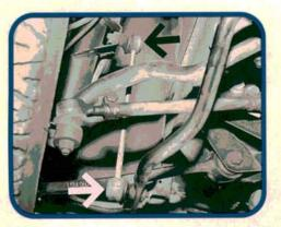
Under the car, check the stabilizer links for wear or binding. Some will groan a warning, others simply pop apart. Also check the thrust rod bushings which take an awful beating, especially during braking. To replace them, remove the thrust rods and press out the old bushings.
