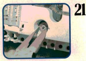
Remove the 5.5 mm screws (a 7/32 socket will work in a pinch) holding the fuel and temp gauges, and the washers below them. Then use needle nose pliers or a similar tool to unscrew the round slotted nuts below the washers. Alternately push the two studs on the gauge assembly until it pops out of the board.
