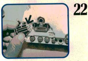
When you get down to bare SI boards, lay them side by side and transfer all bulbs, hole for hole. Use the BMW bulb removal tool or needle nose pliers. Twist the bulbs into the new sockets. Also transfer the coding plug to the new board (arrow). Squeeze the tabs on the sides of the plug and pull it off.
