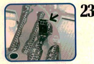
The new board comes with a small bridge connector which must be installed on the two tiny pins below the tach. Do this before you reinstall the tach. This connector powers up the new board and readies it for use. There should be an instruction sheet inside the box with the new board.
