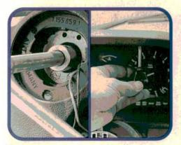
Remove the steering wheel (22 mm socket). Lay a soft towel over the steering column so you don't scratch the face of the cluster. Remove the two small Phillips<sup>™</sup> screws at the top of the cluster, and gently pry down on the top of the cluster housing as you tilt it toward you away from the dash.
