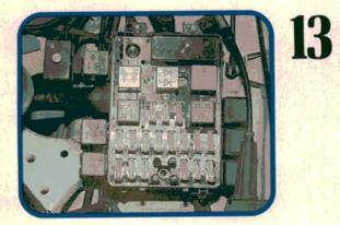
Check for corroded connections at the main and fuel pump relays mounted next to the fuse box (or Power Distribution Box as BMW calls it). Intermittent main relay voltage drops can be a real joy to track down. Also check fuses for clean, tight connections.
