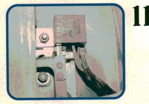
An absent minded door lock heater control unit can stay on and burn out the door lock heater for the driver side door lock. This control unit sits next to the door handle linkage in the driver's door. If the unit stays ON (and the coil hasn't burned out yet), the outer door skin will get hot to the touch.
