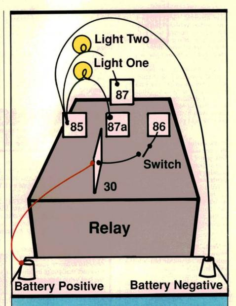
Our diagram shows how to wire your relay socket for both four and five terminal relays. The five terminal relay is different from the four terminal in that it isn't a simple ON/OFF circuit like the four terminal. Instead, as the relay coil goes on or off in the five terminal relay, a switch contact toggles between terminals 87 and 87a. That means that there is continuity between 30 and 87a with the relay coil off. There is continuity between 30 and 87 with the relay coil energized.
