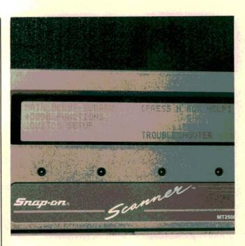
4 After making our connections and turning on the ignition key, the scanner recalls the stored VIN and asks if we're still working on the same vehicle. We answered "Yes" and headed for the Main Menu. The menu lists the diagnostic functions available for our test car. We'll check Code Functions first.
