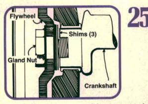
Crankshaft end play is one of the most critical measurements you'll make on this overhaul. End play is set using 3 shims placed between Number 1 main bearing and the flywheel. Do this before installing jug sets. That way you don't fight the added friction when sliding the crank fore and aft.
