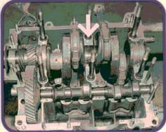
We have chosen to use Loctite 518 as our case half sealer, (no blue glue please). We final check for burrs on the sealing surface and apply a thin, thin film to the case half sealing surfaces. We also install a new rubber sealing ring (arrow) on each case stud. We're ready to assemble the case.
