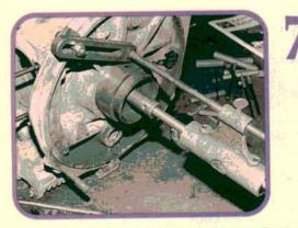
It wasn't easy to find line boring equipment here in Akron. But Dave Zakikian jumped at the chance to dust off his old line boring tool and give us a hand. The case wasn't all that bad, and a first oversize cut (0.50 mm) cleaned up the bores. We ordered firstover bearings with a standard thrust.
