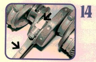
Rods are installed on the crankshaft so the boss on the neck of the rod (left arrow) will point upward when the crankshaft assembly is in the case. Rods and rod caps have matching numbers stamped on them. You can't get the caps on backwards unless you're really determined to do so (right arrow).
