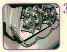
Rocker shaft assemblies are often overlooked during an overhaul or valve job. All of the oil passages in our rocker arms were coked shut. Oil from the lifters passes through the hollow push rods to lube the rocker arm pivots. We clean the shaft assemblies and replace the lash adjustment screws which are shot.
