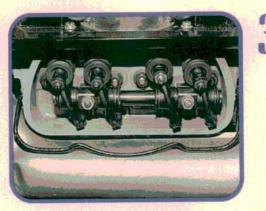
Since the heads hold everything in place (jugs, push rods, heater boxes, muffler, etc.), head torque is critical. This newer style case has stud inserts and is less apt to "pull studs" from the case. Make sure all threads are clean and lightly lubed. Then install the rockers and adjust the valves (cold) to 0.15 mm.
