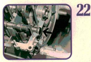
We're almost ready to put the case halves together. Cam and crank are installed, the distributor drive gear is in place. Don't forget to install the cam plug (arrow) or you'll have a massive oil leak. Apply a thin film of sealer to the plug and drop it in place. We check to make sure everything is turning freely.
