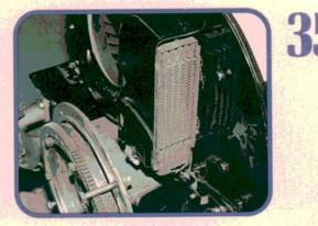
An oil cooler acts like a small radiator to remove excess heat from the engine's puny  $2^{1/2}$  quarts of oil. Early style oil coolers were mounted inside the fan housing and partially blocked the flow of air to Number 3 cylinder. This later style engine mounts the cooler on an offset mount to correct that problem.
