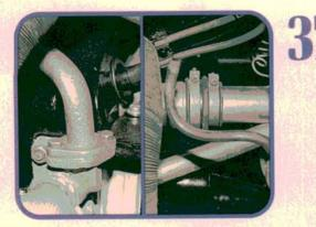
Intake manifold tips. A cross tube runs across the base of the intake manifold and bolts to the muffler. Heat from the exhaust warms the intake to prevent icing in winter. Make sure the tube isn't plugged with carbon. Also check the rubber boots on the intake for cracking which will cause a big vacuum leak.
