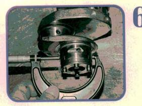
The thrust face of the case is okay. But we've estimated that we'll need to line bore the case and install larger OD bearings. Our crank journals are within specs for diameter, and none are out of round. Bearings are available in both over- and undersized thicknesses for case cutting and crank grinding.
