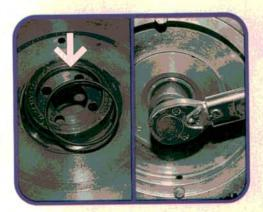
The crankshaft seal fits into a groove in the flywheel. Pry out the old seal (arrow), and install a new one. Reinstall the flywheel, and lock it so it won't turn. Final torque the gland nut (don't forget the big washer that goes under it) to 343 Nm (a whopping 253 ft-lb). Final check end play (0.07-0.13 mm).
