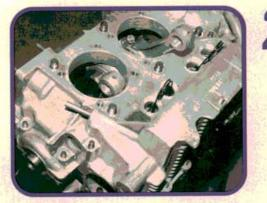
Install the other half of the Number 2 bearing in the remaining case half. Guide the rods through the cylinder holes as you lower the case half. Snug the nuts on the main case studs. With the nuts torqued to spec, everything still spins free. Tighten the 8 mm nuts and bolts around the case perimeter.
