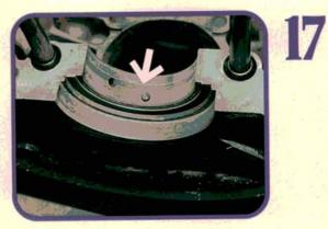
There are locator dowels in one side of the case for each main bearing to keep them from spinning. When you install the crank assembly in the case, be careful to properly index each bearing so its dowel hole fits right over the dowel. Get the holes out of index and you ruin the bearing and lock up the crank.
