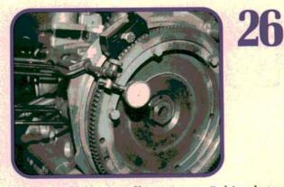
Setting end play. Install two "starter" shims between the flywheel and crank and tighten the flywheel gland nut. Set up a dial indicator on the flywheel as shown. Once you measure total end play with two shims, subtract 0.07-0.13 mm (0.025-0.080 inch). This tells you how thick the third shim needs to be.
