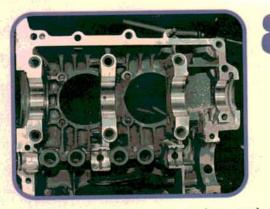
Our case journals come out clean and shiny, but there are chips everywhere. We'll spend some extra time here making sure the inside of the case is spotlessly clean. That includes cleaning all the coke from the oil passages and making sure the oil pickup is clean and fits tight in the case.
