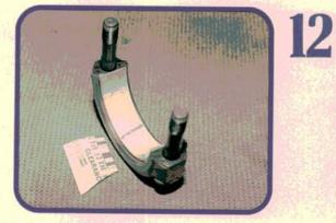
Rods. We already used a micrometer to check the rod journals, and a dial bore shows that standard rod bearings will do the trick. We use a plastic clearance checker, just to be sure. Once installed, the rods should turn smoothly without binding. In fact, installed rods should fall smoothly from their own weight.
