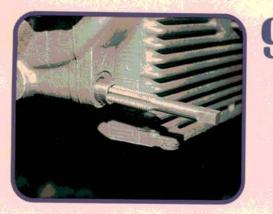
This later style case has two oil pressure reliefs, one which controls oil pressure to the mains, and one which limits oil pressure to the oil cooler. Both of the oil relief pistons are stuck. We screw a 10 mm tap into the pistons to remove them, and clean and polish until both move freely in the case.
