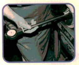
Over at the bench we check piston diameters and cylinder bores. Things go well until we get to the last jug which has a nasty taper and is out of spec for out-of-round. If the case and crank check out, we decide that a new jug set is probably the best way to go. The rings are shot anyway.
