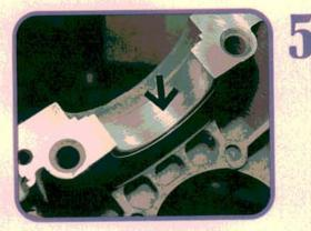
The four main bearing crank likes to thrash around in the aluminum case. Main bearing wear may not be your only problem on a high miler. This case shows signs of the pounding the bearing has given to the case bores. Number 1 main is also the thrust bearing. Wear to the case bore and thrust surfaces can result.
