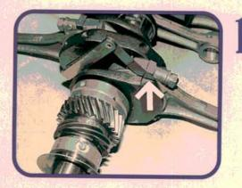
We press in new piston pin bushings and hone them so each new piston pin slides through snugly, but smoothly. We also check rod axial clearance (arrow) and find we're still at the original spec. Too much axial play can result in oil consumption problems when too much oil is thrown against the cylinder walls.
