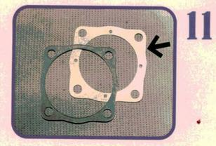
Be careful to install the pump gaskets in the correct order. The thicker of the two goes between the pump body and engine case. The thinner gasket (arrow) goes between the pump body and pump cover. Reverse them and you end up with too much clearance between pump gears and cover, reducing oil pressure.
