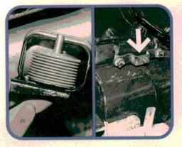
A thermostat mounts to the case below Numbers 1 and 2 to control the air flaps in the fan housing. The flaps stay closed until the thermostat expands and opens the flaps, allowing more air to cool the cylinders. Check all the flaps for free movement before you install and adjust the thermostat.
