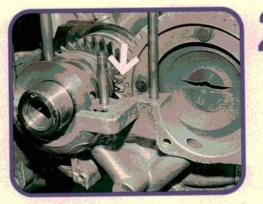
Prelube the lifters and drop them into the case. Install the cam and crank. Timing marks on crank and cam align as shown. Check the backlash between the cam drive and driven gears. Look for zero backlash to a maximum of 0.050 mm. Replacement gears are graded by gear pitch to allow adjustment of backlash.
