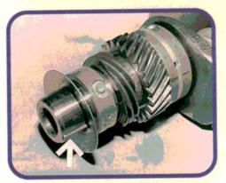
Don't press the gears back on. Make sure the crank area where the gears ride is burr free. Heat the gears in an oil bath (about 180 degrees F) and slide them onto the crank. The timing mark on the cam drive gear faces the slinger. Reinstall the snap ring, Number 4 bearing, oil slinger, and woodruff key (arrow).
