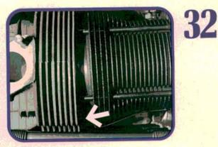
The push rod tubes are squeezed between the head and case as the heads are torqued. That means they want to push the head outward at the bottom at first (arrow). Tightening the bottom row of head nuts first seats the cylinders squarely in the heads.
