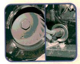
The engine is air cooled by a fan bolted to the back of the alternator (or generator). ALL sheet metal must be installed and properly fastened for the cooling fan to do its job. Even the rubber boots on the spark plug wires must fit properly or valuable cooling air will be lost (right photo).
