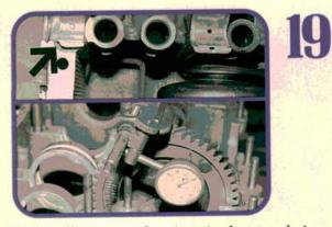
We install new cam bearings in the case, being careful not to swap the two bearings shown. Note how the narrower bearing shell does not block the oil return passage in the case (arrow). Then we check camshaft end play (bottom photo). The new bearings do the trick, and our end play is within specs.
