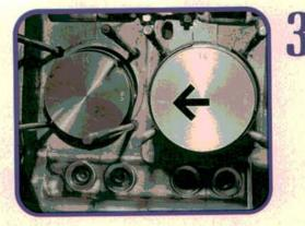
Piston pin bores are slightly offset from the centerline of the piston. As a result, they must be installed with the arrow on the piston head pointing toward the flywheel. Pistons pins are held in place by snap rings (two per piston) which fit in grooves in the piston pin bores.
