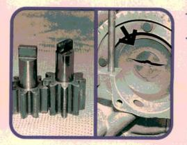
Our engine also has the later style, larger capacity oil pump with taller gears. The use of the deeper pump meant a change in camshafts. The face of the newer cam is slightly dished to accept the taller pump (right photo). Our old pump is worn out. A new one is cheap insurance.
