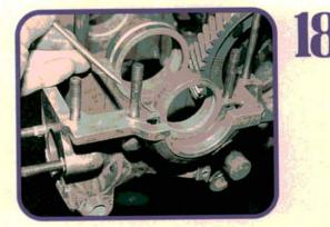
One way to be sure the bearings are properly positioned is to install the bearings in the case without the crank. Then take a tiny scribe (a dental pick in this case) and gently mark each bearing for index. Install the bearings on the crank and use the scribe marks to position them as you lower the crank assembly into the case.
