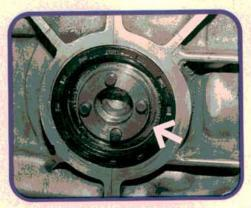
Remove the flywheel, install a shim of the thickness determined in the last step. Reinstall the flywheel and double check end play. If everything's okay, remove the flywheel one more time and install a new flywheel seal. This photo shows the shims peeking out from behind the new seal (arrow).
