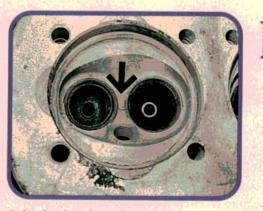
Cylinder head work was always a money maker on these. Cracks in the heads were a common problem, especially cracks near the plug hole, and between the valve seats. We'll weld the cracks and install new seats. These heads are certainly usable, although some will be beyond repair.
