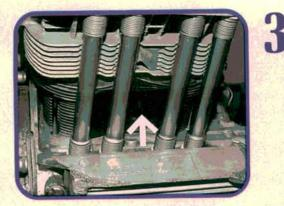
With the jug sets installed, snap the air deflectors into place below the cylinders (arrow). We install new push rod tubes and seals and make sure they're properly seated between the head and case. Push rod tube seams should point upward. The tubes should measure about 191 mm from seal to seal.
