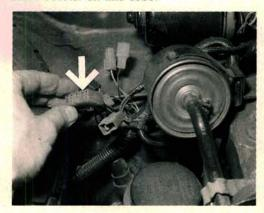
A larger diagnostic connector is located either under the hood near the green test connectors, or below the steering column near the control unit, depending on model year and fuel system. Four different self-diagnostic modes are available. Scan tools can also be used to retrieve serial data on injected models.
