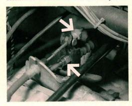
Hill Holder and clutch free play adjustment can be confusing the first time around. Just remember that if the clutch cable is loosened, you'll need to tighten the Hill Holder cable by an equal amount. A properly adjusted Hill Holder will release the brakes just as the clutch begins to engage.
