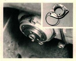
One camshaft support bolts to the front of each camshaft case. The o-rings that seal the supports to the cases may cause oil leaks in this area. Engine heat causes the o-rings to harden and compress. We replaced the o-rings and lip seals at both camshaft supports to prevent future oil leaks.
