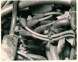
An engine knocking noise that sounds like it's coming from the distributor could be caused by a loose left timing belt. Pushing on the distributor may change the pitch of the noise. The loose cam belt causes the camshaft drive gear and distributor driven gear to chatter against the camshaft drive gear.
