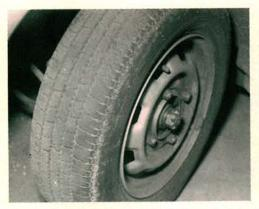
Regular tire rotation is especially important on 4WD models. Uneven front to rear tire wear may cause 4WD engagement/disengagement problems. Tires must be the same number size and diameter (a good reason for replacing tires in sets of four). Unequal tire diameters will also cause accelerated tread wear on On Demand systems.
