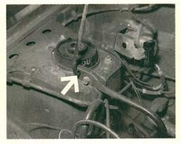
The two position hood is a handy feature. Move the hood prop from its core support location to the mounting eyelet located at the right strut tower. Install the other end of the prop in the secondary hood notch. This raises the hood to a nearly vertical position for easy accessibility.
