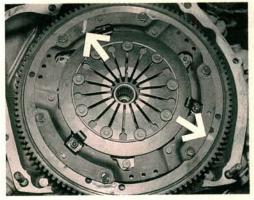
The pressure plate must be properly indexed during clutch service. The flywheel and pressure plate have painted balance marks along their outer edges (arrows). Do not line up these balance marks. Instead, install the pressure plate with the marks 120 degrees away from one another.
