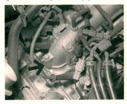
The aluminum engine parts expand and contract during heating and cooling cycles. Special gaskets are used between the intake manifold and the cylinder heads to handle these size changes. Do not apply sealer during manifold gasket replacement, as this will cause premature gasket failure.
