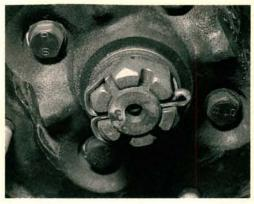
Front wheel bearings will wear out quickly if the hub nut is not properly torqued. Always tighten the hub nut to the recommended torque setting during rotor or drive axle service. If the castle nut slots don't line up, the nut may be tightened up to an additional 15 degrees.
