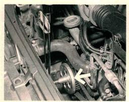
Rotate the crankshaft three times before adjusting belt tension (engine cold, tensioner bolts loosened). Line up the timing marks, then install a beam type torque wrench and cam sprocket adapter on the cam sprocket. Apply the recommended torque to remove belt slack. Tighten the tensioner bolts while maintaining the torque.
