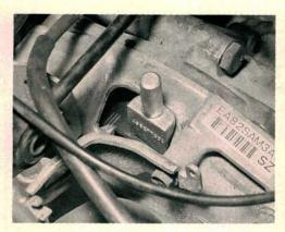
We used this factory flywheel lock to remove and reinstall the crankshaft pulley bolt. The flywheel lock's dowel pin engages a hole in the flywheel. The flywheel timing notches and timing pointer used for timing belt installation and tensioning are visible to the left of the flywheel lock.
