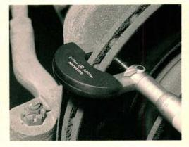
Rotor and drum resurfacing shouldn't be considered mandatory with every pad or shoe replacement. Check for deep scoring, then measure runout, taper, parallelism, or thickness variations. New pads or shoes should work fine if these measurements are still within specifications.
