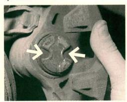
A parts store of our acquaintance had a rash of "bad" Subaru front calipers. It seems the technician who was condemning the parts didn't know that the caliper piston must be turned clockwise to retract it into the caliper. A large C-clamp should not be used to retract the piston.
