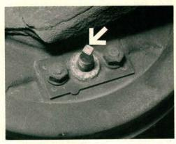
Rear brakes normally last a very long time. The primary shoe gets most of the wear. Rear brakes are manually adjusted on FWD models. Remove the protective boot and turn the square adjuster clockwise to take up for brake shoe wear. Four wheel drive models have self-adjusting rear brakes.
