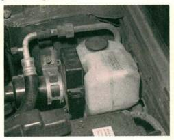
Cooling system maintenance is especially important. Neglected antifreeze can cause internal engine corrosion, blockage, head gasket failure, and cylinder head cracking. Keep the outside of the radiator clean and replace the antifreeze at the recommended intervals (or sooner) to prolong engine life.
