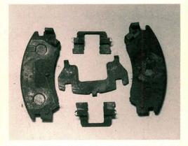
Inspect the condition of all brake hardware during brake jobs. Original equipment and premium front pad kits include new shims and the correct high temperature lubricating grease for the job. Front brake squeak can often be traced to pad hardware that is damaged, improperly lubricated, or missing.
