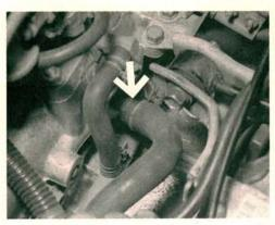
The PCV valve is hidden at the back of the intake manifold and is often overlooked as a maintenance item. A clogged PCV valve may force oil into the intake manifold and foul the air flow meter on 1985-86 port fuel injection systems. This prevents proper air flow meter operation, causing driveability problems.
