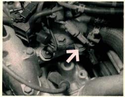
Loose or corroded ground connections may cause fuel injection problems. Engines with single point injection have an important ground next to the thermostat housing (arrow). Port fuel injection engines have a ground at the intake manifold. Additional fuel injection harness grounds are located on the core support.
