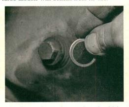
The oil pan drain plug washer should be replaced each time the drain plug is removed. A reused washer loses its ability to seal the threads. Overtightening the drain plug to keep it from leaking risks stripping the pan threads or rounding off the drain plug hex. A new washer is cheap insurance.
