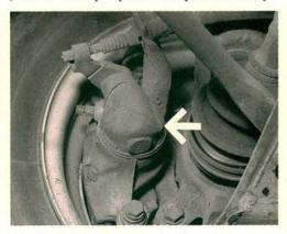
The front calipers include the parking brake mechanism. At the same time you are checking the CV boots for tears, check the rubber parking brake boots at the back of the calipers. Torn caliper boots will leak lubricating grease and let water in, preventing proper parking brake operation.
