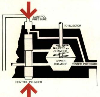
Here's a cutaway view of a fuel distributor. An internal passage allows system pressure to reach a chamber above the control plunger. This pressure pushes the plunger down in its bore. The greater the pressure above the plunger, the more vacuum it takes to lift the sensor plate. Less pressure above the plunger makes it easier for the sensor arm to lift the plunger. The same amount of vacuum at the sensor plate lifts the plunger higher, richening the mixture. And a cold engine needs more fuel.
