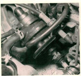
If the VCM control vacuum signal drops low enough to open the vacuum sensors, look for broken or disconnected vacuum hoses between the VCM and the ISCA, or between the ISCA and the vacuum switches. An internal ISCA diaphragm failure is a third, but less likely possibility. The vacuum switches provide the ground to the vacuum cut solenoids and are wired in series. A break in the switch wiring or a failure of either vacuum switch will also open the vacuum cut solenoids.
