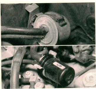
You'll see opposite effects if either the VCM or ISCA air filters get clogged. A clogged VCM air filter causes a high VCM control vacuum signal to the ISCA. This retracts the ISCA push rod, slowing hot and cold idle speeds. A clogged ISCA air filter causes a high idle at all times. Outside air must pass through the ISCA's internal air bleed to weaken the manifold vacuum signal and retract the ISCA push rod. Test the system after removing the filter hoses if you suspect a clogged filter.
