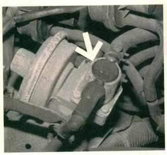
A stuck VCM can prevent the ECU from controlling idle speed. An air filter near the VCM must remove any dirt or water from the air before it enters the VCM to create the control vacuum signal. Weak filters caused moisture damage to early VCMs, making them stick. The ECU's duty cycle signal should make the VCM tick rapidly while the engine is running. Replace the VCM if it's stuck. Hitting a stuck VCM may revive it temporarily.
