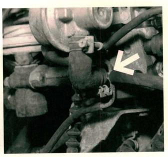
The whole idle speed control system runs on vacuum, so a strong manifold vacuum supply is a must. The VCM gets its manifold vacuum from a vacuum port at the back of the intake manifold, below the carburetor. The vacuum port is also near the EGR valve, which may clog the port with carbon. A low manifold vacuum supply to the VCM, caused by a clogged port or leaking vacuum hose, will weaken the VCM's control vacuum signal to the ISCA. This will cause a high or hunting idle after engine warm up.
