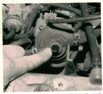
If the engine has no cold fast idle, your first inclination might be to look for an adjustment screw. I've seen several perfectly good ISCAs ruined by cranking on this adjustment screw or by turning the ISCA push rod. This adjustment screw and a smaller one on the carburetor linkage control maximum idle speeds. But they seldom need adjustment unless someone has gotten to them before you. We'll show you several more likely causes for no cold fast idle you should check first.
