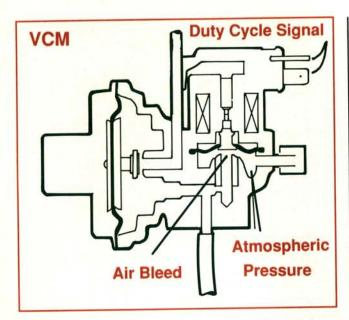
The ECU uses the Vacuum Control Modulator (VCM) and Idle Speed Control Actuator (ISCA) to control idle speed at all engine temperatures. A variable air bleed inside the VCM mixes outside air with manifold vacuum to translate the ECU's duty cycle signal into a control vacuum signal. When the engine is cold, the ECU's duty cycle signal to the VCM is high. The VCM translates this into a weak control vacuum signal to the ISCA to increase cold idle speed.
