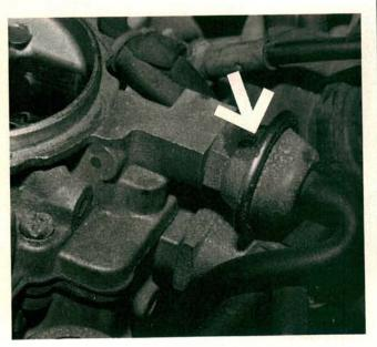
The Vacuum Piston does the job of a choke unloader on a conventional carburetor. Low manifold vacuum during cranking lets the Vacuum Piston extend, blocking an air bleed between the bowl and the Richer Solenoid to allow full enrichment. Full enrichment isn't needed after the engine starts. Higher manifold vacuum opens the Vacuum Piston, exposing the air bleed to limit enrichment and emulsify the fuel. Vacuum Piston failure will cause an over-rich mixture during warmup.
