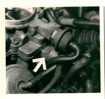
There's no choke plate to limit the supply of air during cold operation, so extra fuel must be added instead. Based on information from the coolant sensor, the ECU sends a varying duty cycle signal to the Richer Solenoid. When the Richer Solenoid needle opens, fuel flows from the bowl to an opening below the secondary throttle plate. A failed Richer Solenoid can cause cold engine stalling. A leaking solenoid needle will cause a rich mixture after warmup.
