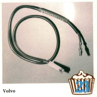
This patch harness can repair a Volvo 7-Series which starts but floods and stalls at temperatures below 25 degrees F. Remove the blue/green wire from the plug at the cold start injector. Snip off the end of the wire and insulate the bare end by taping back against the carside harness.
