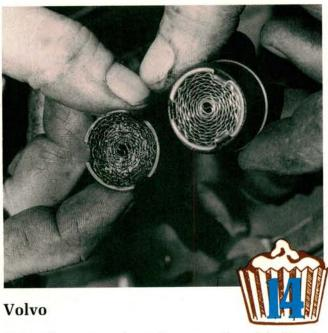
Volvo flame traps have been mentioned before in these pages. Acting as a crankcase breather restriction, they can get so plugged that the crankcase can't breathe. If your Volvo customer can't get the oil leaks stopped, it may be because crankcase pressure is forcing oil past seals and gaskets.
