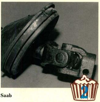
There are two universal joints in the Saab 900 steering column. The one outside the firewall can rust and bind over time and lead to "steering by Armstrong." Some steering racks have been mistakenly blamed and replaced before the real cause of the problem was discovered.
