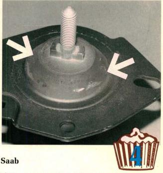
These newer style hydraulic Saab motor mounts are used on 9000s and late model 900s. They will fracture over time in the general area shown by our arrows and leak oil. A bad mount may be more noticeable in a 900 when drivetrain torque produces a noise, and causes excessive shifter movement.
