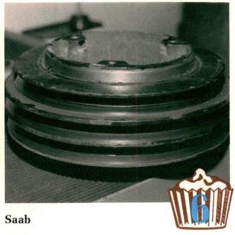
Harmonic balancers on Saab 900s are hidden down low, out of sight. If you hear a scraping or grinding noise from that area, check the balancer. The outer ring can separate from the rubber connecting it to the inner hub. Then it walks toward the engine until it starts grinding away at the front cover.
