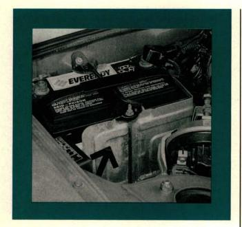
It's plenty hot under the 300's low hood. Batteries can have a shorter than normal service life as a result. Battery shields on later models deflect some of the heat. Replacement batteries may be shorter than the original. Install the available spacer below the battery for proper mounting.
