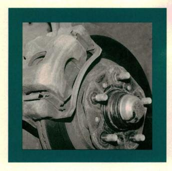
Rotor thickness variations caused brake pulsation problems on some 300's. Factory "countermeasure" rotors that are machined to closer production tolerances (0.0005 mm) are available to correct this problem. These rotors should not be turned before installation. Most brake lathes can't match this accuracy.
