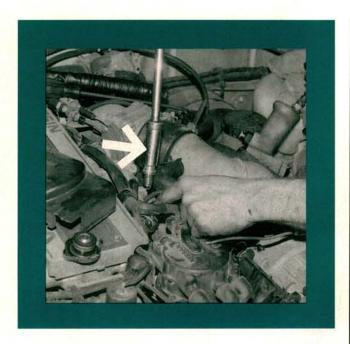
Changing the spark plugs can be a challenge. This swivel socket with attached extension helps a lot. Road dirt and other unfriendly debris may settle in the recessed areas around the spark plugs. To avoid internal engine damage, clean these areas with compressed air before removing the plugs.
