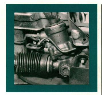
Power steering rack leaks have been a common occurrence on 300's. If the rack shaft seals are leaking, the boots will be filled with fluid. Visually inspect the rest of the rack for leakage. Use care when installing the hose fittings, the aluminum housings will crack or cross thread very easily.
