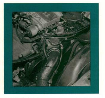
6 Timing belt replacement is an important preventive maintenance service at 60,000 miles or sooner. This engine can bend internal moving parts in an expensive fashion if the belt breaks. We've also heard reports of head bolts breaking, then jamming the camshaft and stripping the timing belt.
