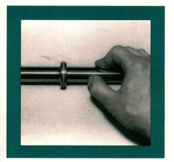
Rack repair or replacement is a judgement call. Replacement parts are available if you go the repair route. Installing new seals with worn rack parts will guarantee a comeback. Run your finger nail over the rack shaft. Even a small amount of rack shaft wear will cause seal leakage later.
