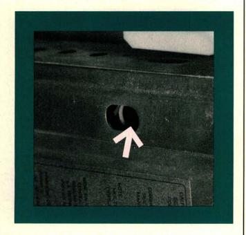
The ECU's green diagnostic LED can be used to monitor oxygen sensor activity. Warm up the engine, then maintain 2000 RPM for about two minutes. A good oxygen sensor should flash the green LED at least 10 times in 10 seconds. Fewer than 10 flashes indicate a lazy oxygen sensor that should be replaced.
