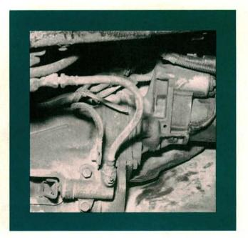
Transmission removal and clutch replacement doesn't get much easier than this rear drive setup. To avoid hard shifting complaints, always use the correct lube in manual transmissions. Many complaints (especially in cold weather) are caused by using the wrong gear lube instead if the specified 75W-90 or 80W-90.
