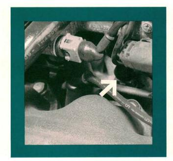
5 The injectors are buried under the intake plenum. Injector harness connector corrosion can be a problem, especially in humid climates. The connectors may look fine, but even a small voltage drop can cause an intermittent miss. Solder all connections and use shrink wrap when replacing connectors.
