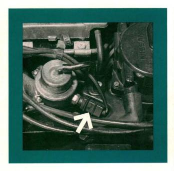
This sensor in the fuel pressure regulator monitors fuel temperature. During hot restarts, the ECU closes the pressure regulator control vacuum solenoid valve to raise the fuel pressure and prevent vapor lock. This system wasn't 100 percent effective on 1984 models and was modified on later models.
