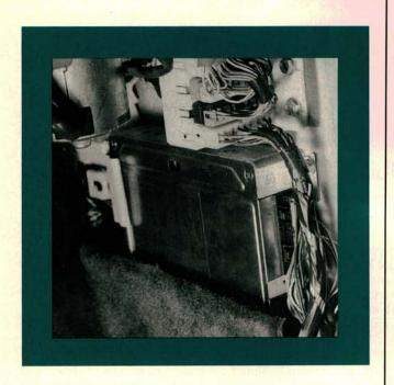
The ECCS control unit is hidden behind the right kick panel trim. The diagnostic LEDs can be seen through a small hole in the trim, but you'll need to remove the trim if you want to access trouble codes or change to any of the five diagnostic modes without the aid of a scan tool.
