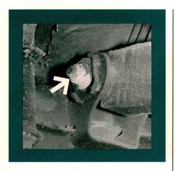
19 Front and rear toe are the only adjustable alignment specifications. Rear toe is adjusted by turning this eccentric bolt at the inner pivot point of the lower control arm. Weak rear springs can affect ride height and will cause camber and toe changes and accelerated rear tire wear.
