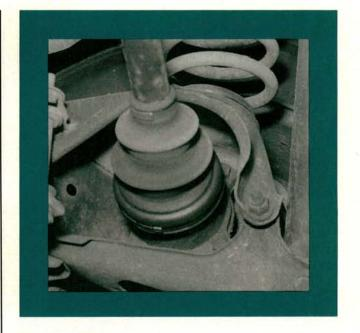
A clicking noise from the rear during acceleration and deceleration may have two different causes. Worn rear CV joints are responsible in some cases. The spacer between the inner and outer wheel bearings may also shift and click. An updated axle flange and revised torque specifications were introduced to correct this problem.
