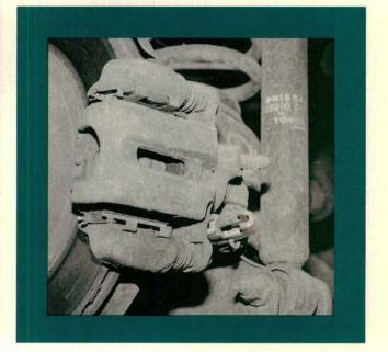
Dragging brakes may also be caused by a caliper parking brake mechanism that is binding internally. Disconnect the parking brake cable. If the caliper lever now moves freely, the cable is to blame. If the lever still doesn't release completely, the problem is inside the caliper.
