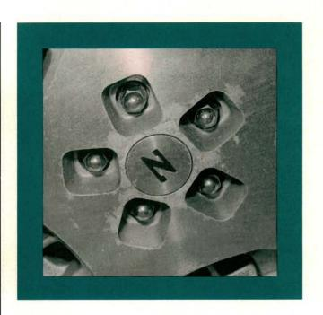
Start the lug nuts by hand, then tighten in a diagonal pattern to avoid cross threading, wheel damage, and rotor warpage. The alloy wheels are centered by the lug nuts, not the hub flange, so the lug nuts must be tightened alternately and evenly to center the wheel. Finish the job with a torque wrench.
