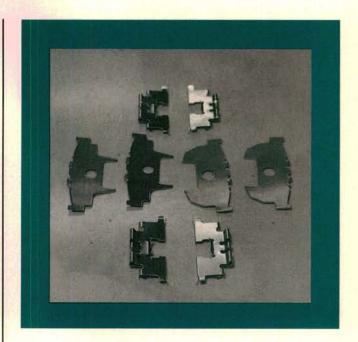
The condition of front and rear brake hardware can have a big effect on brake noise. Brake shims get rusty and disappear in cold weather states. Worn rear brake slide pins will cause a rattling noise over bumps. The noise goes away if you apply the brakes slightly. Slide pins are not available separately.
