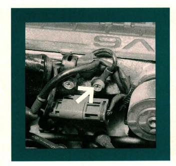
Electrical problems aren't as common as you might expect for a car with so many accessories crammed into such a small area. An important ECCS grounding terminal is located at the corner of the intake manifold (arrow). A loose or dirty connection here can cause rough running and stalling at idle.
