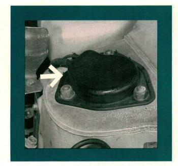
Rear shocks seem to wear out and leak more quickly than the front struts. The rear suspension may bottom over large bumps after the fluid leaks out. The electrically adjustable struts and shocks (arrow) on turbo models can be very expensive to replace. Always support the rear suspension before removing a rear shock.
