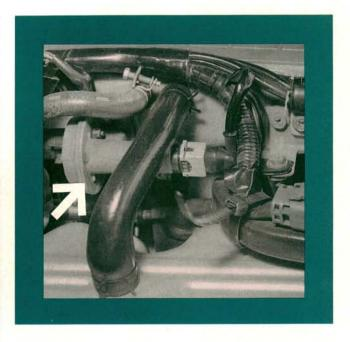
A sluggish cold air regulator will cause a low idle speed when cold. The engine may also load up and stall due to the extra cold enrichment. The regulator must open so air can bypass the closed throttle plate. Cleaning the valve seldom helps. A weak bimetal spring is usually to blame.
