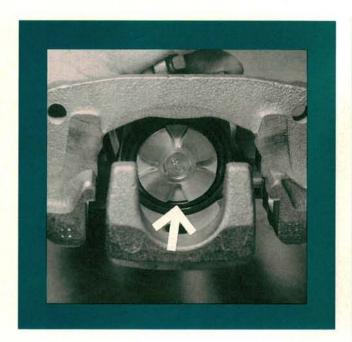
15 Before new rear pads can be installed, the caliper pistons must be turned clockwise to retract the pistons into the calipers. Check behind the dust shield before turning the piston. Rear calipers may begin to leak after piston retraction if the seals are weak or the pistons are rusted.
