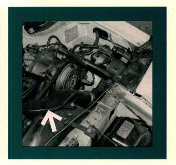
High underhood heat can also cause hot restart difficulty. Fuel containing alcohol seems to aggravate the restart problem. Later models use a bottom feed injector design to prevent vapor lock and fuel boiling. The injector cooling fan (arrow) on turbo models also helps.
