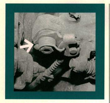
Make sure the parking brake mechanism operates smoothly. Binding parking brake cables accelerate rear brake pad wear. There should be 0-3 mm clearance between the rear caliper parking brake lever and the stopper pin when the parking brake is released. Rusted cables are common.
