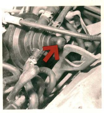
Restart the engine, then remove the rubber plug from the top of the ISCA. Adjust the ISCA screw to obtain an idle speed of 1500-1900 RPM in neutral for both manual and automatic transmission models. Shut the engine off, then reconnect the water temperature sensor and turn the ECU diagnostic switch off.
