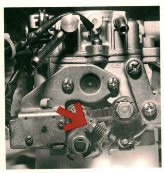
Raise the engine speed to 2000 RPM. The DVOM should read 0 volts. Slowly lower the engine RPM. At 1200 RPM, the DVOM should read 12 volts. Bend the linkage tab to adjust the throttle switch on earlier carburetors. Later carburetors have an easier to use threaded adjuster. Recheck your adjustment.
