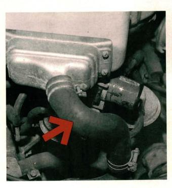
To adjust the CO, run the engine until it reaches operating temperature, then let it idle for two minutes. Disconnect and plug the air induction hose at the air cleaner. Rev the engine to 2-3000 RPM two or three times, then return to idle speed. The warm idle speed must be below 1000 RPM.
