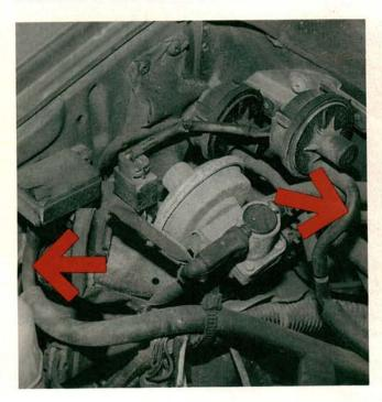
The ISCA adjustment is our next stop. Disconnect and plug the boost sensor vacuum hose. Disconnect the vacuum hose from either of the vacuum switches. Leave this hose unplugged. Disconnect and plug the vacuum hose leading from either of the vacuum cut solenoids to the air filter.
