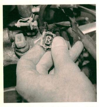
Shut off the engine, reinstall the vacuum hoses, then move the ECU diagnostic switch to the "ON" position. Locate the water temperature sensor at the rear of the intake manifold and carefully remove the sensor's harness connector. Bridge the connector terminals with a jumper wire.
