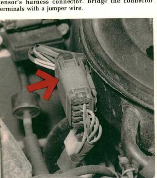
An incorrectly adjusted or sticking throttle switch may cause a hesitation while driving. To adjust the throttle switch, connect the positive lead of your voltmeter to the green wire with white tracer on the carburetor side of this connector. Ground the voltmeter's other lead.
