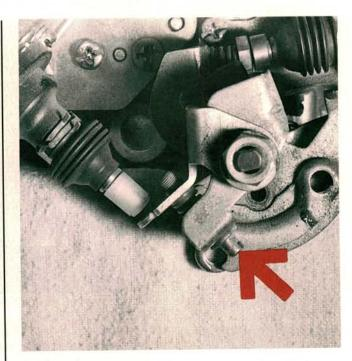
Start the engine and be ready to work quickly. Adjust the small screw at the bottom of the car buretor throttle shaft bell crank for an idle speed of 2800-3200 RPM for M/T and 3200-3600 RPM in neutral for A/T. Adjusting toward the low end of the spec is easier on the engine's bottom end during cold starts.
