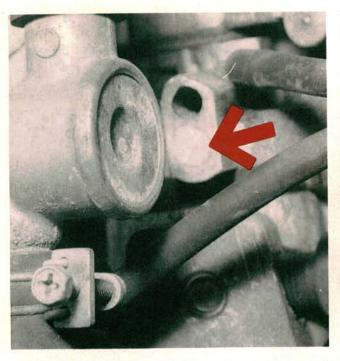
Restart the engine and rev to 2-3000 RPM several more times before returning to idle speed. Check the idle CO percentage and adjust if necessary by turning the idle mixture screw. Stop the engine, reconnect the air fuel ratio solenoid harness connector, then disconnect the VCM harness connector.
