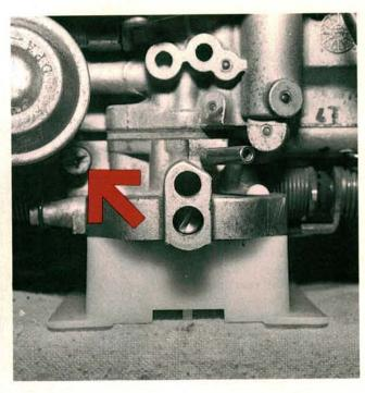
Restart the engine and rev to 2-3000 RPM several more times before returning to idle. Check the base idle speed and adjust if necessary, using the small screw at the base of the carburetor ( $700 \pm 50$  RPM for M/T,  $550 \pm 50$  RPM in Drive for A/T). Stop the engine and reconnect the VCM harness connector.
