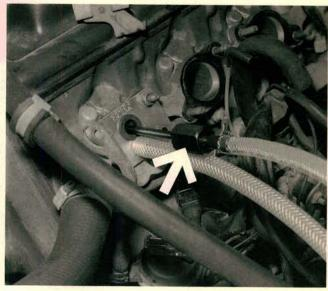
Unless your arms are extra long and you can do two things at once, have an assistant turn the blaster's red knob to the "ON" position while you hold the blast nozzle in the port plate grommet. Inlet air pressure must be maintained at 60-80 PSI. The blaster uses lots of air, so inlet pressure may drop while you clean.
