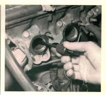
Before you go any further, move the blast nozzle around inside the port to get a feel for where the valve stem is located. This will help you do a thorough cleaning job by feel alone. You won't be able to see what you are doing when the intake port plate is installed.
