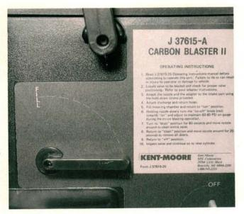
A lever on the side of the blaster casing dumps a pre-measured amount of shell material into the blast chamber. One turn of the lever to the "FILL" position should give you enough crushed walnuts to clean one intake valve. Return the lever to the "RUN" position before you begin blasting.
