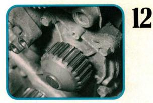
Depending on the vehicle mileage, the water pump may fall into the "while you're at it" category. The pump is driven by the timing belt and would sure mess up the new belt if the pump decided to leak a short time later. A seized pump could also cause internal engine damage. It's your decision.
