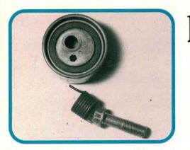
We cleaned the tensioner and checked its condition. We also cleaned the tensioner mounting surface on the block to assure free tensioner movement. The tensioner spring's longer tab fits into the block. The spring moves the tensioner, but final belt tension is adjusted by turning the tensioner hex.
