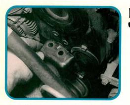
After all six mount bolts are removed, there's just enough room to remove the engine half of the mount. Slowly raise the engine until the other half of the mount can be removed from the body. Take the mount to the bench, remove the rubber end caps, and check the mount for signs of wear.
