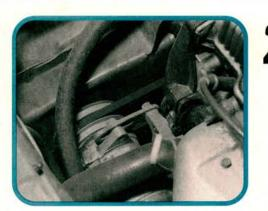
Remove the accessory drive belts. With the splash panel out of the way, it's a clear shot to the lower pivot bolts for the A/C compressor and alternator. The belts came off easily after loosening the upper adjustment bolts. Our Spectrum didn't have power steering to contend with.
