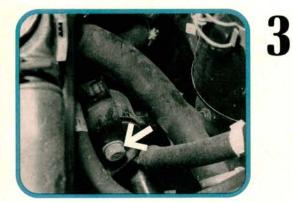
Remove the torque rod located at the rear of the engine, below the air filter snout (arrow). Removing the torque rod lets us raise and tilt the engine without binding the other engine mounts. Both torque rod mounting bolts have captive nuts, so there's no need for a backup wrench.
