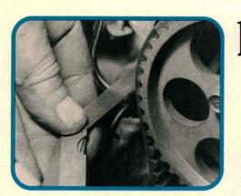
Line up the cam and crank sprocket timing marks. We used a feeler gauge blade edge to recheck the cam sprocket timing mark. Belt tension must be adjusted by feel because there is no room for a belt tension gauge. Tension is properly adjusted when the long side of the belt can be twisted a quarter turn.
