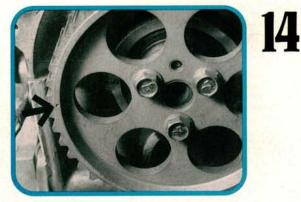
The same goes for the camshaft seal. You won't get an easier chance to replace it. Torque the cam sprocket bolts to 10 Nm (86 in-lb), then line up the small dot on the camshaft sprocket with the top surface of the cylinder head (arrow). The cam sprocket dowel pin should still be at 12 o'clock.
