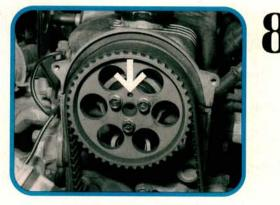
Temporarily reinstall the crankshaft pulley bolt. Turn the crankshaft clockwise until the camshaft sprocket's dowel pin (arrow) is at 12 o'clock. The crankshaft sprocket's keyway should also be pointing straight up. Now we're ready to remove the old belt.
