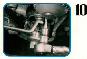
Loosen the twelve point belt tensioner bolt. Relieve the timing belt tension either by pushing on the long side of the belt, or by rotating the spring loaded tensioner clockwise using an Allen<sup>®</sup> socket. Tighten the tensioner bolt, then remove the old timing belt.
