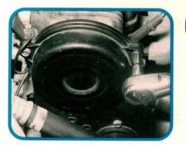
The timing belt cover can be removed either before or after the crankshaft pulley is removed. If you want a quick look at the timing belt or if you're only replacing the water pump, remove the cover now. The bottom of the one piece cover will just clear the crank pulley after the cover bolts are removed.
