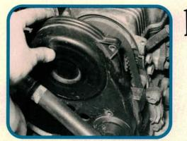
Torque the tensioner bolt to 50 Nm (37 ft-lb), then reinstall the timing belt cover and crankshaft pulley. Lock the crankshaft, then torque the crankshaft pulley bolt to 147 Nm (108 ft-lb). Lower the engine, then reinstall the motor mount bolts, rear torque rod, and drive belts.
