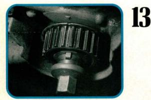
More preventive maintenance. Check the condition of the front crank seal and replace it if necessary. Make sure that any debris from the old belt is cleaned out of the crank sprocket teeth. Line up the crankshaft sprocket notch with the triangle pointer that's cast into the front cover.
