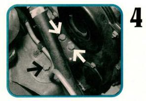
Support the engine under the oil pan with a floor jack and a block of wood. The two piece right side motor mount bolts through the belt cover and must be completely removed. Remove the three upper mount bolts (arrows). Now reach under the mount to remove the three bolts that pass through the belt cover.
