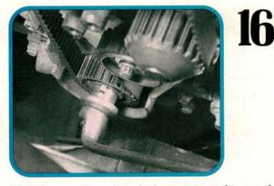
Use the crank pulley bolt to rotate the crankshaft counterclockwise through two complete crankshaft revolutions. This equalizes the belt tension all the way around the belt. It's also a good way to make sure no internal engine parts are going bump in the dark before we crank the starter.
