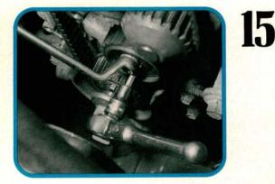
Turn the tensioner clockwise, then tighten the lock bolt. Install the new belt with the manufacturer's name facing you. Keep the slack on the tensioner side of the belt and don't move the camshaft or crankshaft sprocket. Loosen the tensioner bolt to remove the belt slack, then retighten the bolt.
