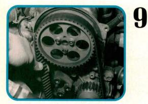
While the old belt didn't look badly frayed after more than 60,000 miles, it had stretched quite a bit. We could twist the belt better than a quarter turn by grabbing the long side of the belt between the crank and cam sprockets. The belt tensioner doesn't adjust belt tension as the belt wears.
