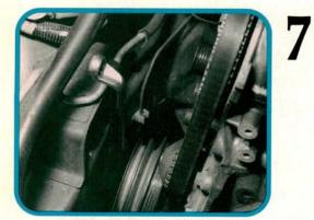
Keep raising the engine until a box wrench or socket will fit over the crankshaft pulley bolt. Dealer service departments have a special tool to lock the flywheel or flexplate. We put the transmission in gear, locked the brakes, loosened the pulley bolt, then removed the crankshaft pulley.
