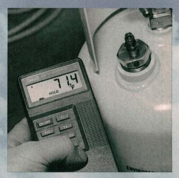
To check for excess noncondensable gas in recycled refrigerant that's stored in a portable container, place the container out of direct sunlight at a temperature of 65 degrees F or greater for at least 12 hours. Measure the temperature within four inches of the container using an accurate thermometer.
