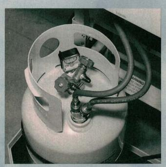
If the refrigerant container pressure is over the allowable limit, slowly vent the vapor from the top of the container into the recycling equipment. Vent until the pressure falls below the limit. If the pressure can't be lowered within limits by venting, the entire contents of the container must be recycled.
