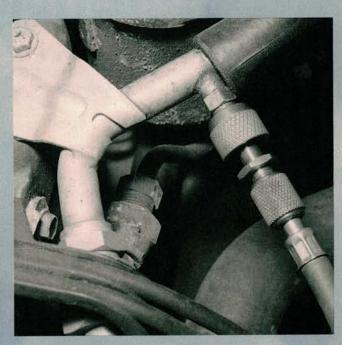
Disconnect the recycling equipment before charging the system, unless it's a recycling and recharging station. All your equipment must have shutoff valves within 12 inches of the hose ends. Use the recycling equipment to draw the trapped R-12 out of the manifold gauge set when you're finished.
