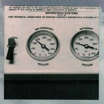
One of the byproducts of recycled refrigerant is noncondensable gas (air). A separate gauge on our equipment measures the pressure of this byproduct. After recycling, we follow the manufacturer's instructions and vent the noncondensable gas to lower its pressure to within 20 PSI of the stored refrigerant pressure.
