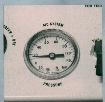
Any refrigerant recovery/recycling equipment you consider should meet UL standards, so equipment from different manufacturers will work in pretty much the same manner. Wait at least five minutes after the machine finishes recycling. If there is still pressure in the system, run the machine through another cycle.
