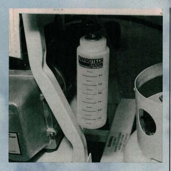
A small amount of oil is pulled out of the car's A/C system during the refrigerant recycling process. Contaminants are also removed with the oil. A bottle on the side of the recycling equipment collects and measures the amount of oil removed so we know how much to add when the system is recharged.
