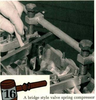
A bridge style valve spring compressor will reach the recessed valve springs and valve seals while the head is installed on the block. The hollow bucket below the tool's lever arm reaches into the well to compress the recessed valve spring. Depress the spring, then remove the keepers with a pocket magnet.
