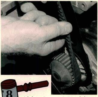
A belt tension gauge isn't needed to set the timing belt tension. Adjust the belt tension by pivoting the water pump counterclockwise. The belt is properly adjusted when it can be twisted about 90 degrees at the midpoint between the camshaft and water pump sprockets. Tighten the water pump bolts to 20 Nm (15 ft-lb).
