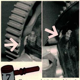
The cam sprocket timing mark is on the back side of the pulley. Line up the mark with the top edge of the cylinder head. The mark is very easy to see with the belt shield removed (left photo). An access window in the belt shield (right photo) allows a glimpse of the timing mark when the shield is installed.
