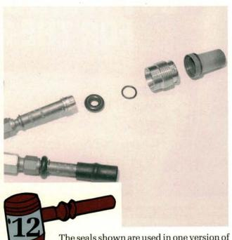
The seals shown are used in one version of the air shroud injector system. The large oring seals the top of the injector to the insert to prevent vacuum leaks. The smaller o-ring seals the tip of the injector. Air enters through the sleeve and must pass through the tip of the injector, rather than around it.
