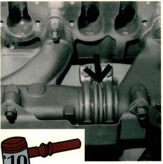
Specially tempered exhaust studs are available for the ports, and should be installed if the original studs break or whenever the exhaust manifold is removed. Replace the self-locking manifold nuts too. This later Audi manifold is jointed between the number 2 and 3 exhaust ports to prevent stud breakage problems.
