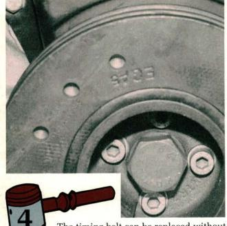
The timing belt can be replaced without removing the crankshaft sprocket bolt. Remove the four Allen bolts that attach the vibration damper to the crankshaft timing sprocket. The sprocket bolt is torqued to 350 Nm (252 ft-lb) at the factory. Add thread locker and you have all the ingredients for a hernia.
