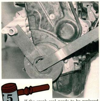
If the crank seal needs to be replaced, leave the vibration damper in place. The tool on the left engages the damper to lock the crankshaft. The tool on the right gives the leverage needed to loosen the crank bolt. If the engine is in the car, brace the damper tool above the motor mount while loosening, and below while tightening.
