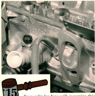
Four cylinder fans will recognize this routine. To replace a valve seal, remove the spark plug and install an air hold to keep the valve from dropping into the cylinder after the valve keepers are removed. Position the piston at BDC to keep the crankshaft from turning when the air is applied.
