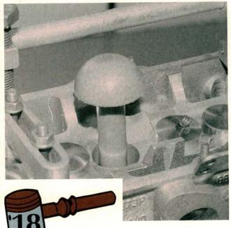
Installing the new valve seal requires one last special tool. This mushroom shaped tool slips over the valve stem and installs the valve seal using hand pressure. Use the small plastic sleeve that's packaged with the valve seals to avoid damaging the new seal as it passes over the valve keeper grooves.
