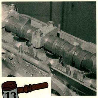
Frequent engine starts and short duration trips may cause hydraulic valve lifter noises. To test the lifters, run the engine until the radiator fan comes on at least once, then raise the engine speed to 2500 RPM. If any lifter noise is still present after two minutes, the noisy lifter should be replaced.
