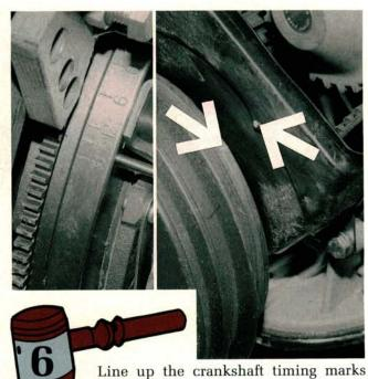
Line up the crankshaft timing marks before installing the new timing belt. If the engine is in the car, use the access window in the bell housing and the marks on the crankshaft (left photo). If the engine is out of the car, use the raised mark on the timing belt cover and the notch on the crank pulley (right photo).
