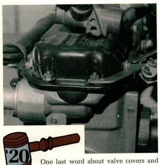
seals. Updated valve cover gaskets using a new rubber gasket material are available to replace earlier cork gaskets which may become brittle and deformed. To prevent oil leaks at the rear of the engine, replace the half moon seal whenever the valve cover is removed.
