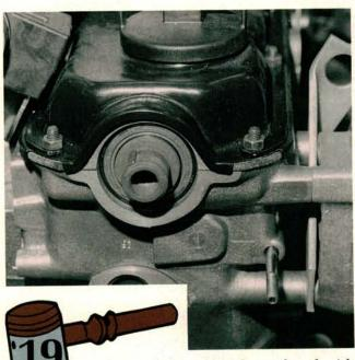
The camshaft seal can be replaced with the cam and valve cover in place, if you have the VW/Audi special tool or are particularly good with a hook style seal puller. It's much safer to remove the valve cover and front cam bearing cap. The seal will slide right out of its groove in the bearing cap.
