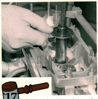
Reaching the valve seal is another challenge. The split collar on this slide hammer tool slips over the outside of the valve seal. Depressing the tool ring tightens the collar around the seal. A quick slap of the slide hammer weight removes the valve seal. Special gripping pliers are also available to do the same job.
