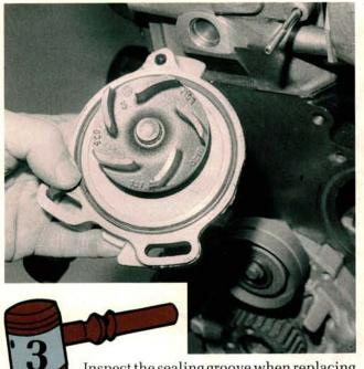
Inspect the sealing groove when replacing the water pump. The grooves on some remanufactured water pumps have been machined to accept a larger 5 mm o-ring. The stock 4 mm o-ring will not seal properly on these pumps. Pumps with modified grooves can be identified by a number 5 stamped on the pump fastening flange area.
