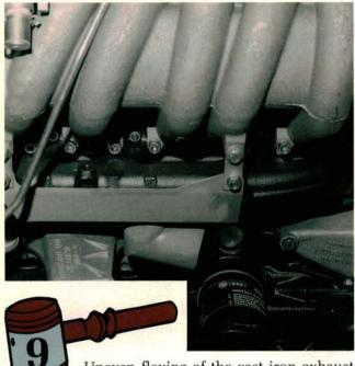
Uneven flexing of the cast iron exhaust manifold may cause exhaust manifold stud breakage at the number 1 and 5 exhaust ports. This Quantum manifold is cast in one piece. Check the manifold's mounting surfaces for flatness. The manifold can be machined to restore flatness and need not be replaced if it becomes slightly warped.
