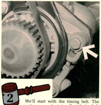
water pump pivots to adjust timing belt tension. There's no intermediate shaft or adjustable idler pulley. Inspect the water pump when replacing or adjusting the timing belt. Always replace the pump o-ring to prevent coolant leaks, even if you're not replacing the pump.
