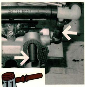
Leaking seals at the air shrouded fuel injectors may cause driveability problems. Metered air is normally diverted from the intake system (right arrow) and routed to sleeves (left arrow) that surround the injectors. The extra air mixes with the injector fuel spray for better atomization.
