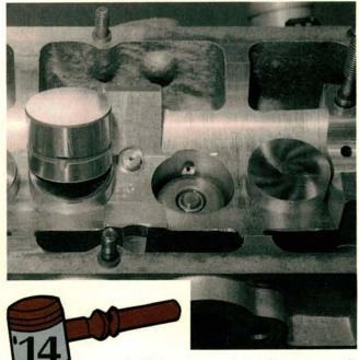
Test the lifters by pushing down on each with a wooden stick, with the valve closed. Replace any lifter that can be depressed. Always store new or used lifters with their cam contact surfaces facing down. Lifters may take 30 minutes to leak down after installation. Don't start the engine during this period.
