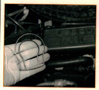
If you are trying to locate the cause of a mysterious loss of coolant, check the condition of the throttle body seal before condemning the head gaskets. Drain the cooling system, then remove the hoses and wiring connectors that are attached to the throttle body. Remove the four throttle body mounting nuts, then lift the throttle body to replace the rubber seal. The seal fits into grooves that are machined into the underside of the throttle body.
