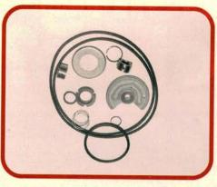
Here's a look at the contents of a typical rebuild kit. As you can see, kits provide replacement for wear items: bearings, seals, and the thrust spacer. If the turbo is so shot that the rotor assembly has turned into a "wear" item, don't chance a rebuild. Turbos which disas-
