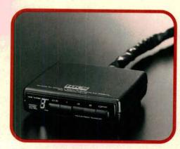
Coke forms at about 330 degrees F. One way to make a couple of extra bucks, and save the turbo, is to install this kit from HKS. Even if the customer shuts off the ignition key, the kit keeps the engine running for 0.5 to 9.5 minutes (depending on temperature) to circulate oil and stabilize exhaust temperatures.
