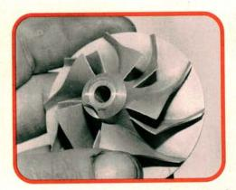
Carefully inspect the compressor and compressor housing for any indications that they've come in contact. The rotor assembly must be properly balanced to withstand speeds over 100,000 RPM. Even the smallest imperfections can cause a catastrophic out of balance condition. And never try to straighten a bent fin.
