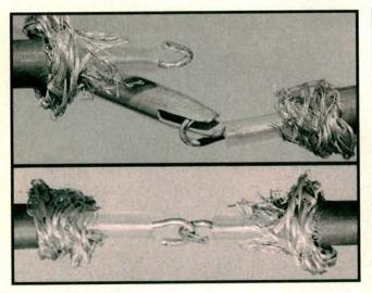
Repair broken shielded cables as follows: Slide a length of heat shrink tubing over one end of the broken cable.
