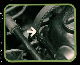
Timing belt replacement procedures are the same as earlier Volkswagen models equipped with the single overhead cam engine. The valves won't bend if the belt breaks, but a broken belt can do some very expensive damage on twin cam and diesel engines. Following the 60,000 mile change interval prevents problems.
