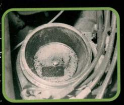
A sludged up valve cover and a clogged PCV system had loaded the top of the sensor plate with an oily residue. We cleaned the sensor plate, then checked for proper centering and height. Adjust plate height by bending the wire spring stop below the plate.
