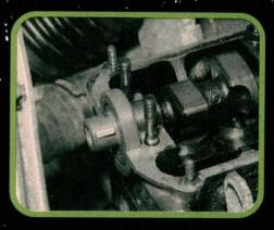
We didn't have the special camshaft seal remover and installer, so we removed the upper half of the camshaft bearing to replace the camshaft seal. The seal sits in a recess at the end of the bearing housing. Once the cam bearing cap is removed, the seal slides right off the end of the camshaft.
