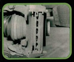
Disc brake noises may occur if brake hardware is missing or in poor condition. A self- adhesive shim kit (P/N 171 698 993) can be installed to correct brake squeak. Make sure the back sides of the pads are clean before installing the shims. Trim any excess shim material before installing the pads.
