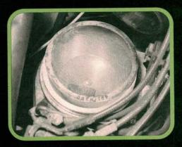
If a KE equipped engine accelerates poorly or lacks power, check for an improperly installed or bent sensor plate screen. A bent or upside down screen will limit the sensor plate's upward travel. Clean and straighten the screen, then install it with the words oben or top facing upward.
